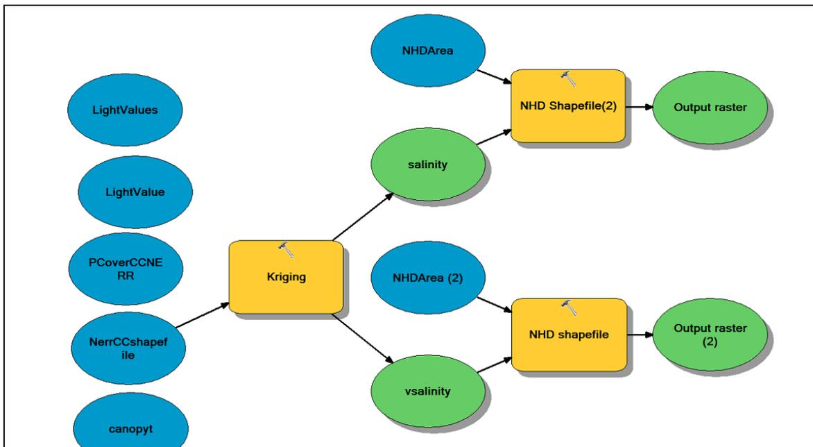
**Figure 2:** Geoprocessing model built using model builder to perform interpolations of all measured parameters.
