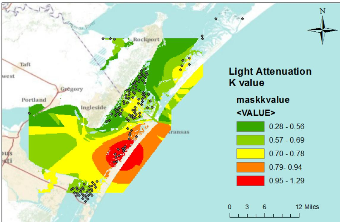
**Figure 10:** Interpolation of light attenuation k values (m-1).
