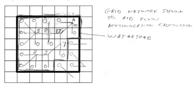
5. Determine a stream network using a **flow accumulation** threshold of 4 grid cells and indicate the grid cells that comprise the stream network. Identify each segment of your stream network using a unique number in the diagram below. You should only fill in stream segment numbers for grid cells on the stream network.
