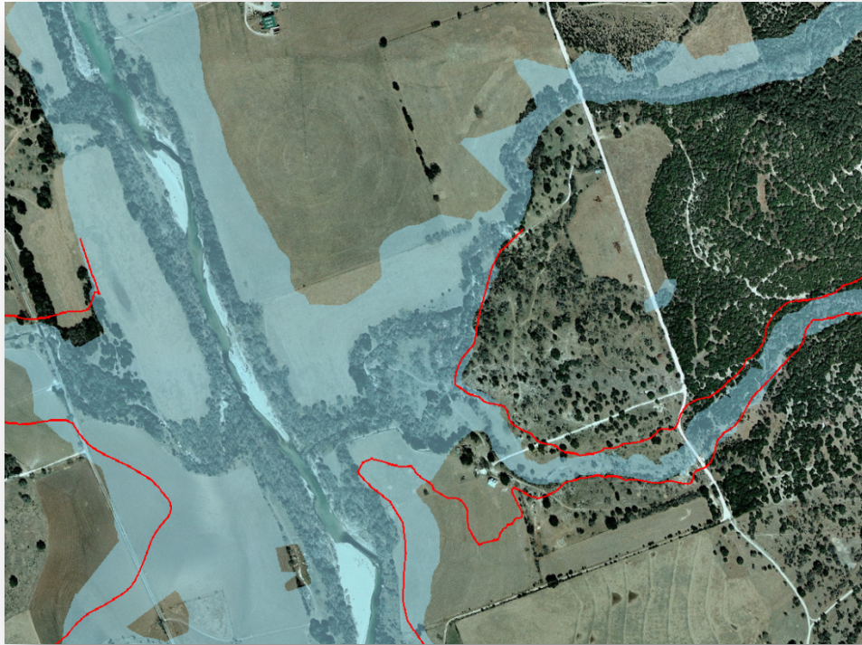
Figure 29: New floodplain map based on the LiDAR terrain (comparing with the FEMA flood extent)
