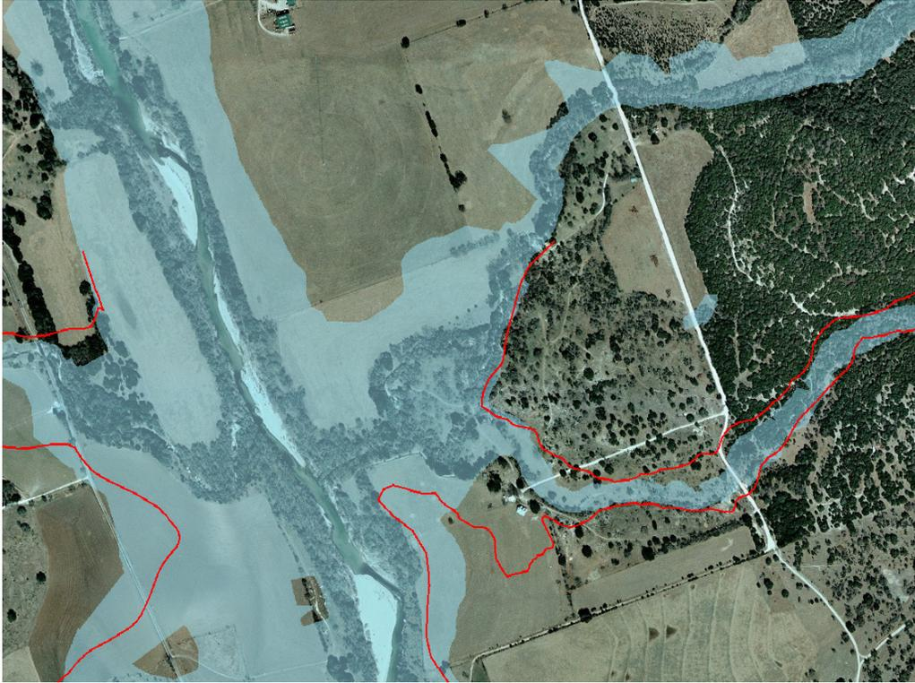
Figure 9: Revised floodplain map with FEMA's 2012 floodplain map superimposed in red lines.
