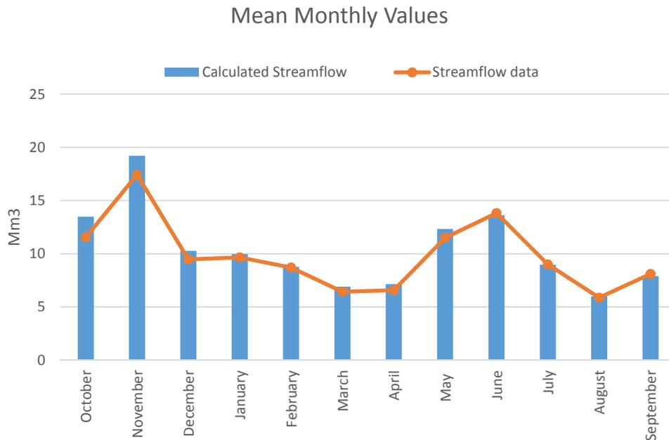
The main differences can be found in October and November. Due to the Mediterranean Climate, major storms occur during these months. These storms are strong in magnitude (mm of rain) and short in duration, making the error between the calculated and the real streamflows larger. For the rest of the months, as said before, the results are quite satisfactory.
