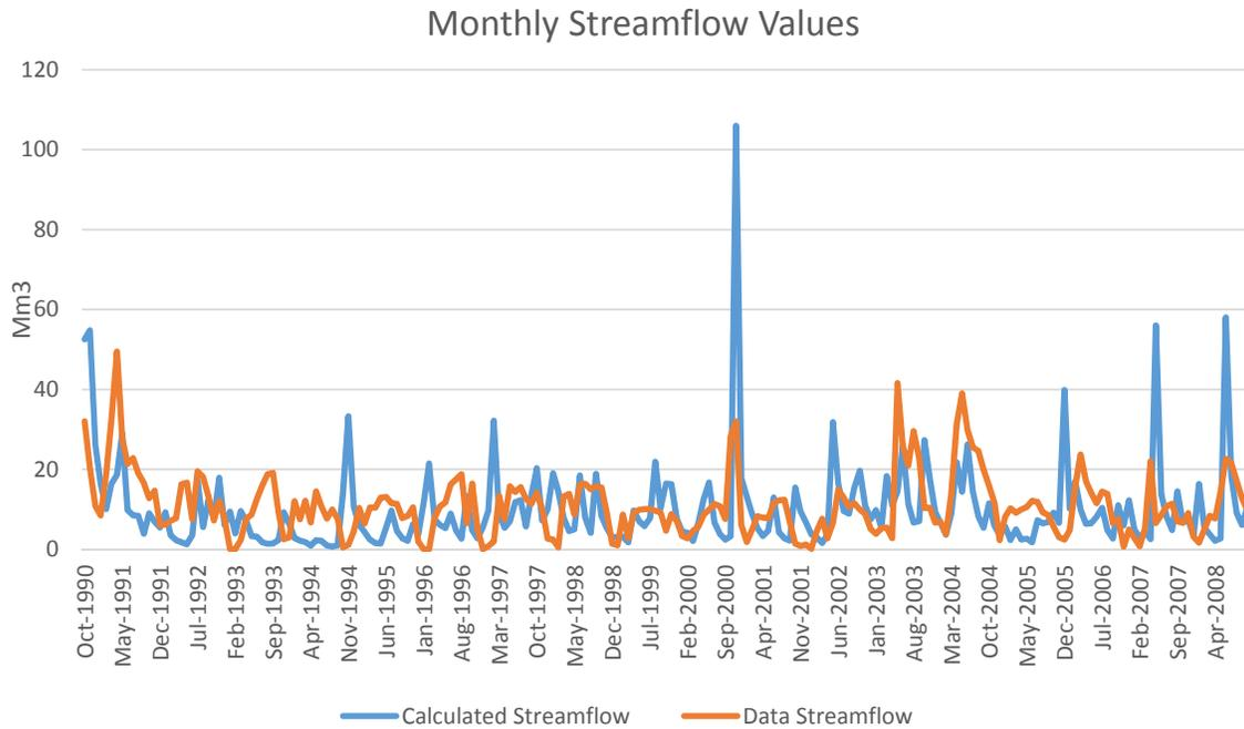
From the Monthly Streamflow Values graph, we can conclude that the model has not yet reached a good calibration, due to the insufficient data available (only from 1990 onwards). The Temez model is primarily developed to model the baseflow and not to simulate well the peak flows. This is evident for October 2000 where the difference in the calculated streamflow and the data streamflow is noticeable.
