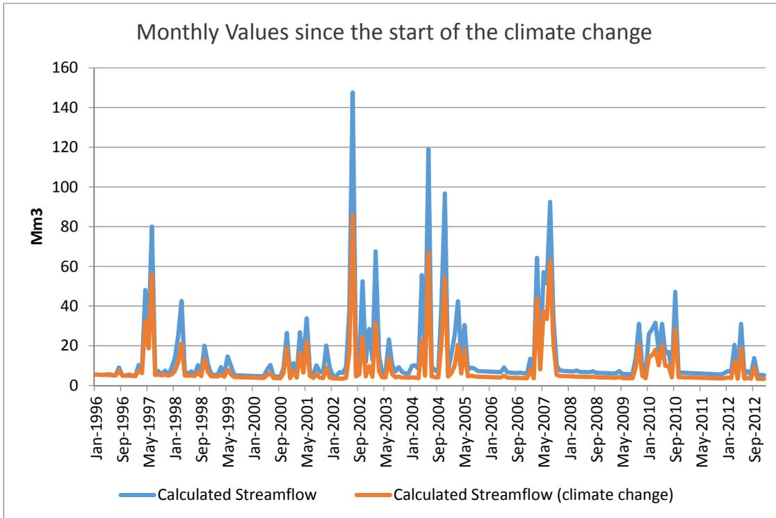
In the above graph it can be observed that the climate change effects in the baseflow (depletion) start to be noticed after, more or less, 2 years of data (1998). The Mean Monthly Values shows us more clearly the importance of the depletion:
