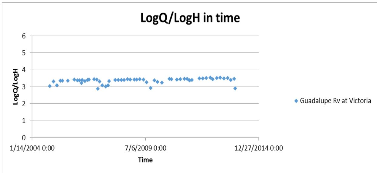
From Figure 7 we can see that we can have a good average from  $\text{Log}(Q)/\text{Log}(h)$  in time. If we analyze other sections of the Guadalupe river and averaged the  $\text{Log}(Q)/\text{Log}(h)$  in time, we have (See Figure 8):
