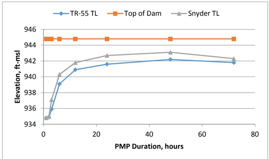
FIGURE 7 - HEC-HMS MODEL WATER ELEVATIONS
