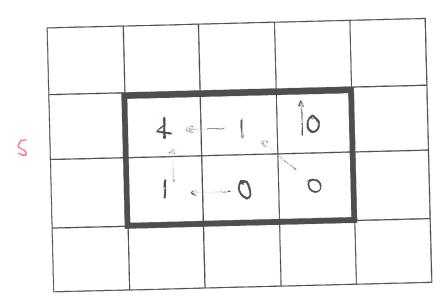
e) Indicate the watershed draining to and including grid cell A by shading the cells included in it. Calculate the area of this watershed in  $m^2$ . Note that you do not need to consider grid cells outside the block of six inner grid cells in calculating the watershed area.
