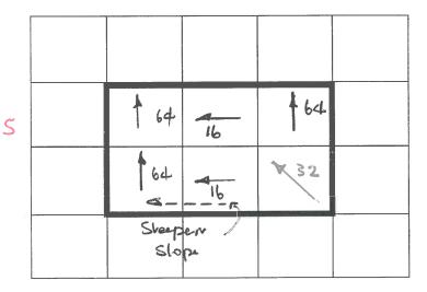
(c) Calculate the Hydrologic (D8) slope of the grid cell with the steepest slope among the six inner grid cells. Indicate which grid cell this is.
