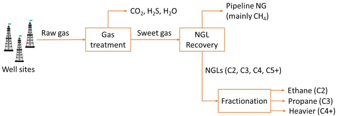
Figure 8. A typical flow in the gas processing plant
