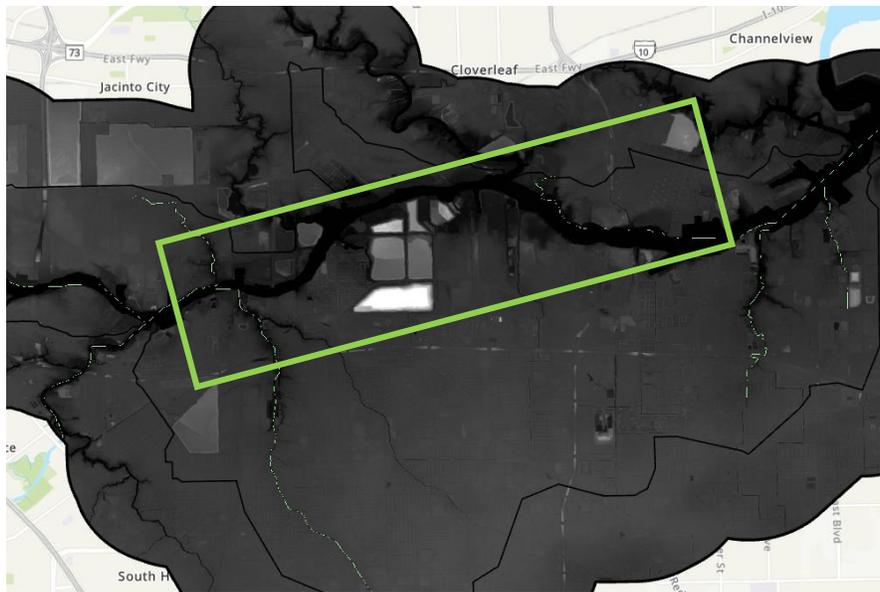
Figure 10 Stream Cut-off in HAND Map
