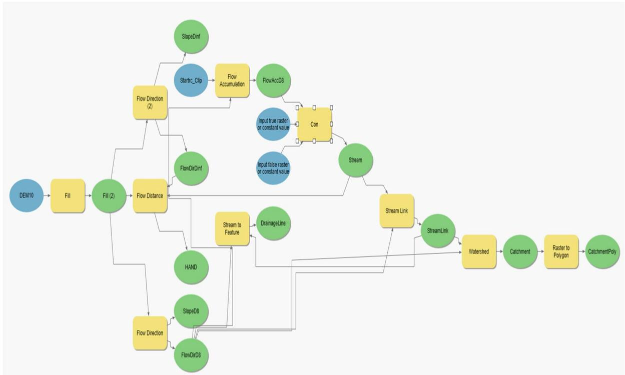
Figure-5: Layout of the model to prepare HAND map
