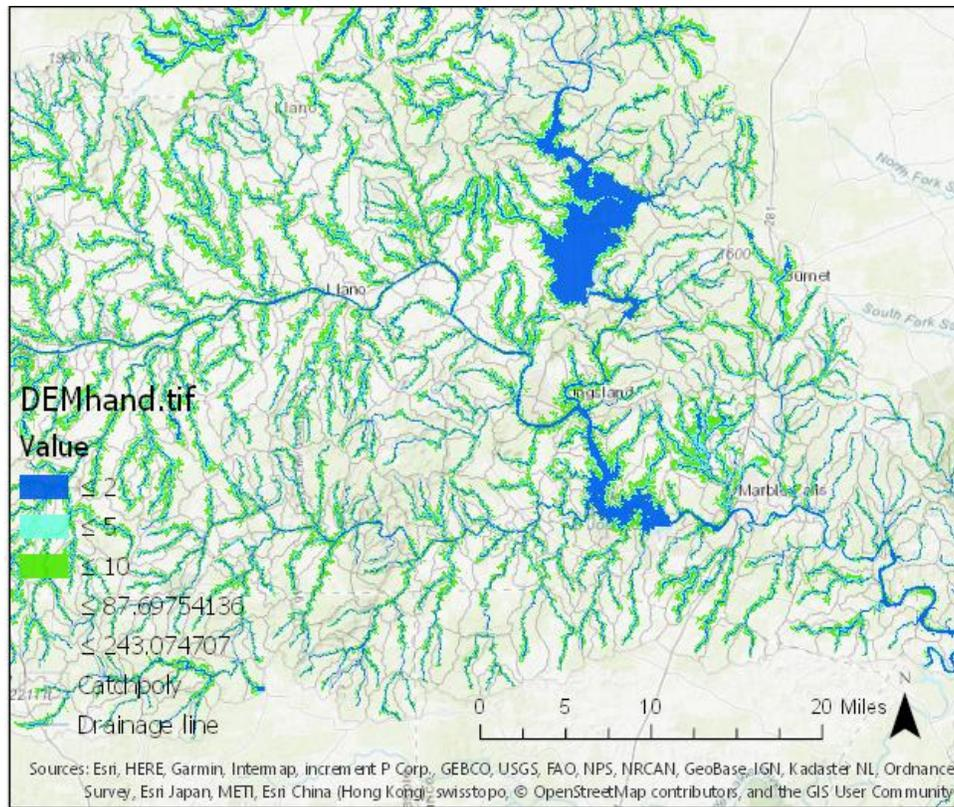
Figure 5. Map showing the HAND raster, drainage line and catchments
