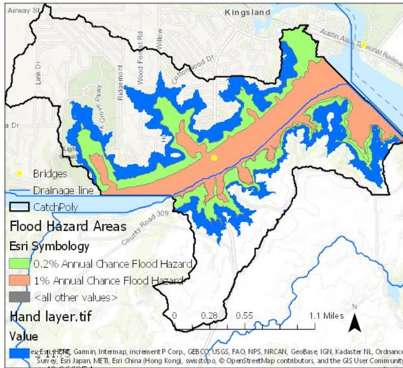
Figure 9. National Flood Hazard Layer and HAND flood depth
