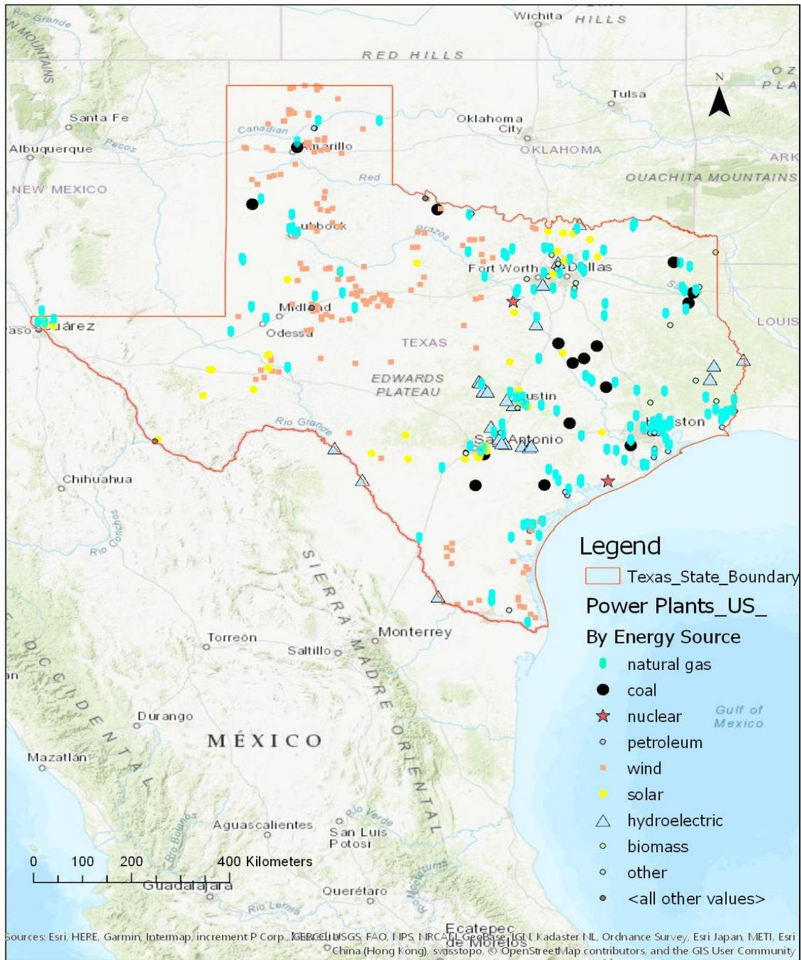
Fig. 3: Map showing the locations of the power plants based on the source of energy they use as the fuel to generate electricity, in the State of Texas.
