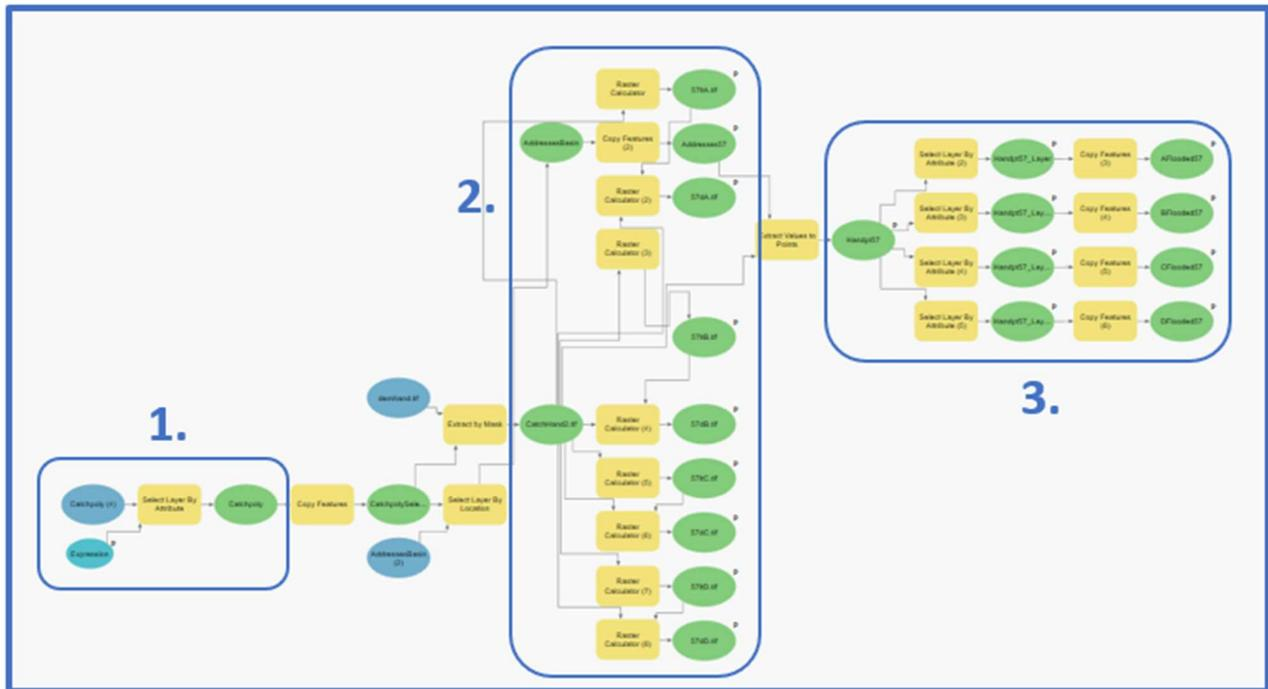
Figure 9: Model Builder used to determine inundation depths and flooded addresses.
