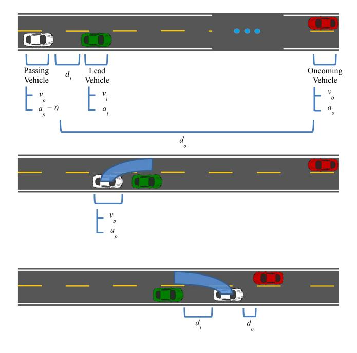
Figure 1. Phases of an Overtaking Maneuver
