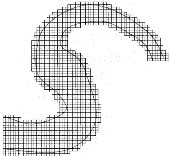
FIG. 1. Channel Bend with Square Cartesian Mesh
