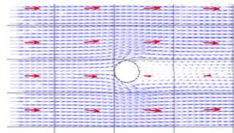
Fig.5. Velocity field filtered to 16 grids
