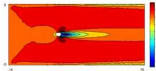
Fig. 3. Local Reynolds number contours around a circular cylinder (white circle) in the computational domain
