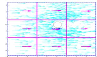
Fig.9. Local and grid-scale mean velocity fields near a circular cylinder with finer and coarser grid cell,  $u_1$  →  $u_1$ ,  $u_2$  →  $u_2$  (in the central cell).
