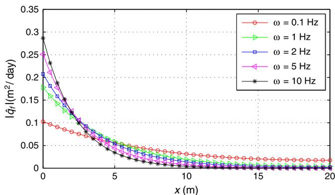
Fig. 11. Leakage rate amplitude versus distance in fracture for wave frequencies  $\omega = 0.1$  Hz to  $\omega = 10$  Hz.
