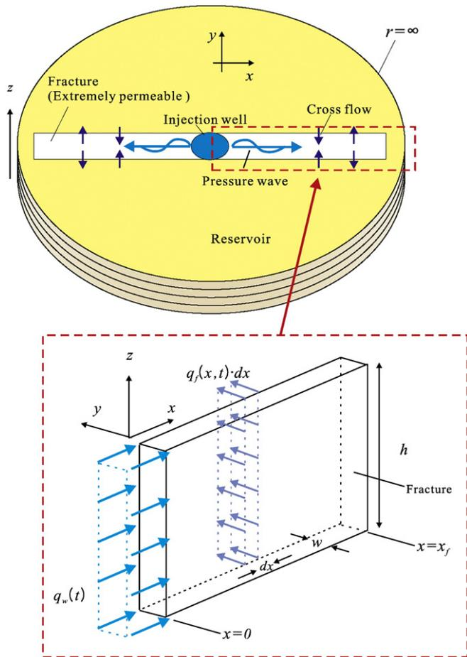
Fig. 9. Propagation of pressure wave in a fractured reservoir. Fluid is injected into the fracture at a rate of  $q_w(t)$ , with fluid leaking through the fracture wall at a rate  $q_f(x,t)$ .
