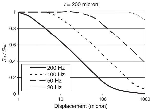
Fig. 8. Residual oil displacement efficiency with respect to the rock displacement and the frequency for a pore radius of 200  $\mu\text{m}$ .
