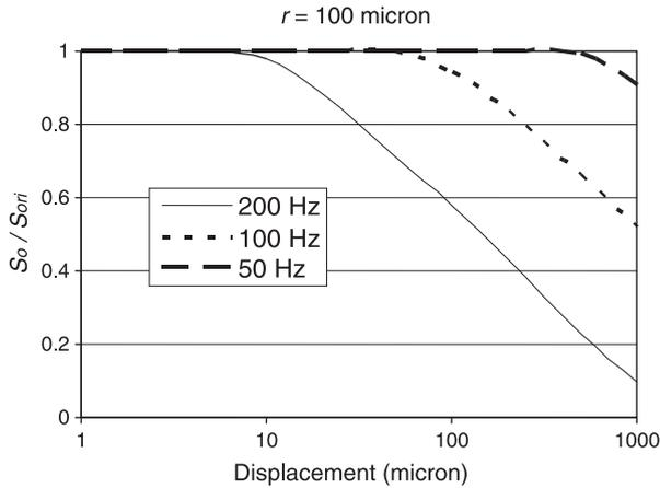
Fig. 7. Residual oil displacement efficiency with respect to the rock displacement and the frequency for a pore radius of 100  $\mu\text{m}$ .
