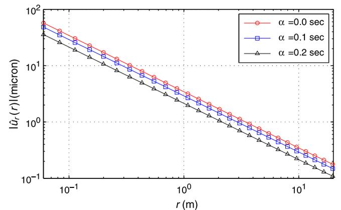
Fig. 6. Modulus of the displacement field of the rock stress wave  $\hat{u}_r(r)$  as a function of distance for several attenuation factors (wave velocity  $c=1000$  m/s, frequency  $\omega=1$  Hz).
