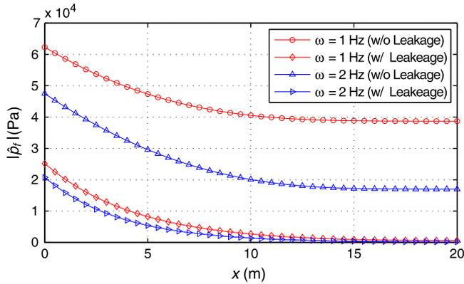
Fig. 10. Pressure oscillation amplitude versus distance in fracture for two frequencies  $\omega = 1$  Hz and  $\omega = 2$  Hz (shown are two cases depending on whether the wall leakage effect is ignored or not).
