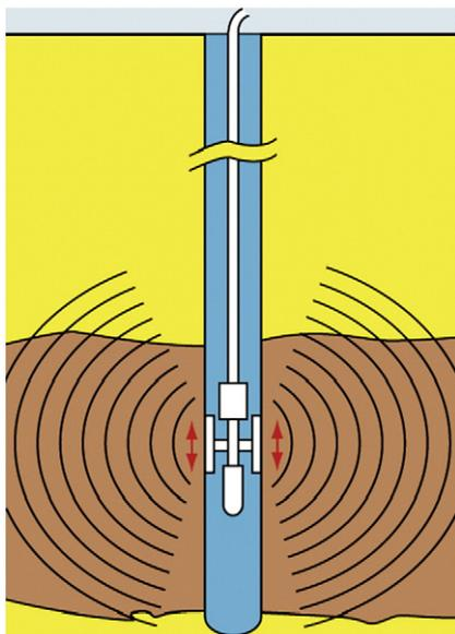
Fig. 1. Schematic of wellbore wave source.
