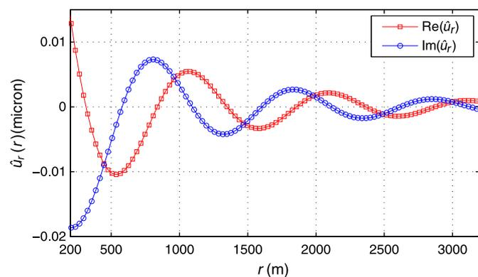
Fig. 4. Real and imaginary parts of the wave amplitude displacement field  $\hat{u}_r(r)$  as a function of distance (rock velocity  $c=1000$  m/s, attenuation factor  $\alpha=0.03$  sec, source frequency  $\omega=1$  Hz).
