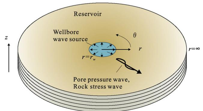
Fig. 2. Wave propagation in a permeable elastic medium induced by a wellbore hydraulic pump wave source.
