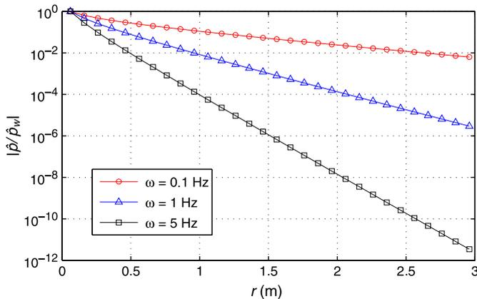
Fig. 3. Modulus of normalized pressure wave  $p_r / \hat{p}_w$  in a homogeneous reservoir–pore pressure solution only as a function of distance from the wellbore source; various excitation frequencies.
