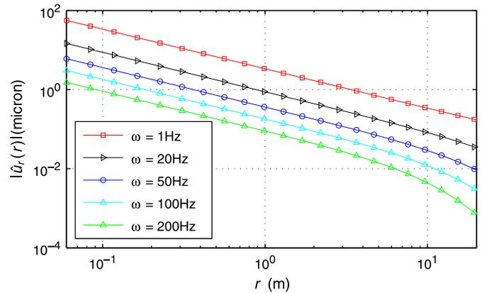
Fig. 5. Modulus of the displacement field of the rock stress wave  $\hat{u}_r(r)$  as a function of distance for several frequencies (wave velocity  $c=1000$  m/s, attenuation factor  $\alpha=0.03$  sec).
