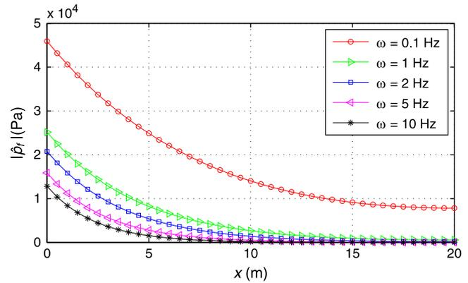
Fig. 12. Pressure oscillation amplitude versus distance in fracture for wave frequencies  $\omega = 0.1$  Hz to  $\omega = 10$  Hz with leakage flow on the fracture wall surface.
