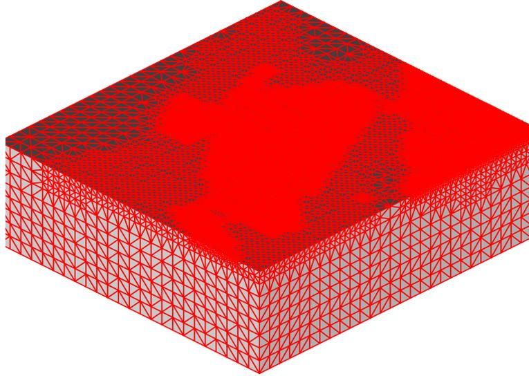
**Figure 3: Tetrahedral element mesh of the San Fernando Valley. Maximum tetrahedral aspect ratio is 5.5. Again, the mesh is much coarser than those used for simulation, for illustration purposes.**
