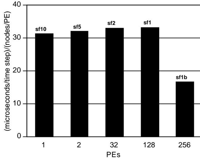
**Figure 10: T3D wall-clock time in microseconds per time step per average number of nodes per processor (PE), as a function of number of processors. This figure is based on an entire 6000 time step simulation, exclusive of I/O. The `sf1b` result is based on a damping scheme in which  $\beta = 0$  in Equation 5 so that only one matrix-vector product is performed at each time step.**
