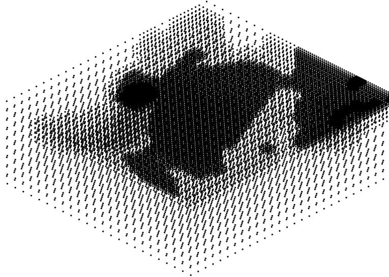
**Figure 2: Nodal distribution for the San Fernando Valley. Node generation is based on an octree method that locally resolves the elastic wavelength. The node distribution here is a factor of 12 coarser in each direction than the real one used for simulation, which is too fine to be shown, and appears solid black when displayed. However, the relative resolution between soft soil regions and rock illustrated here is similar to that of the 13 million node model we use for simulations.**
