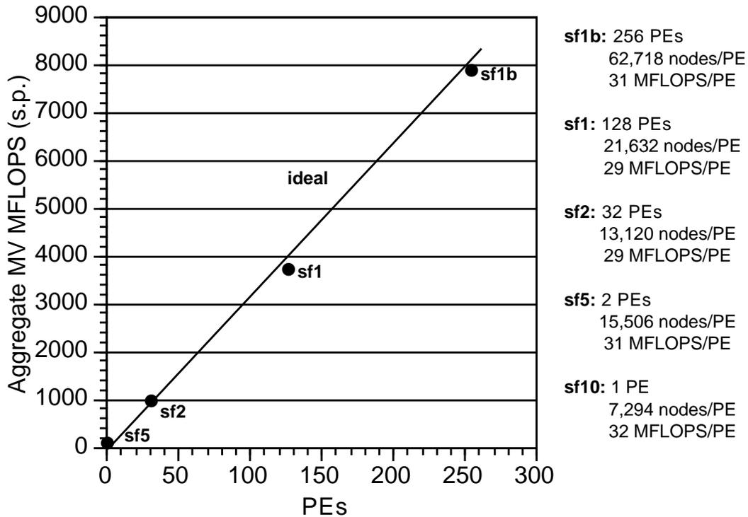
**Figure 9: Aggregate performance on Cray T3D as a function of number of processors (PEs). Rate measured for matrix-vector (MV) product operations (which account for 80% of the total running time and all of the communication) during 6000 time steps.**
