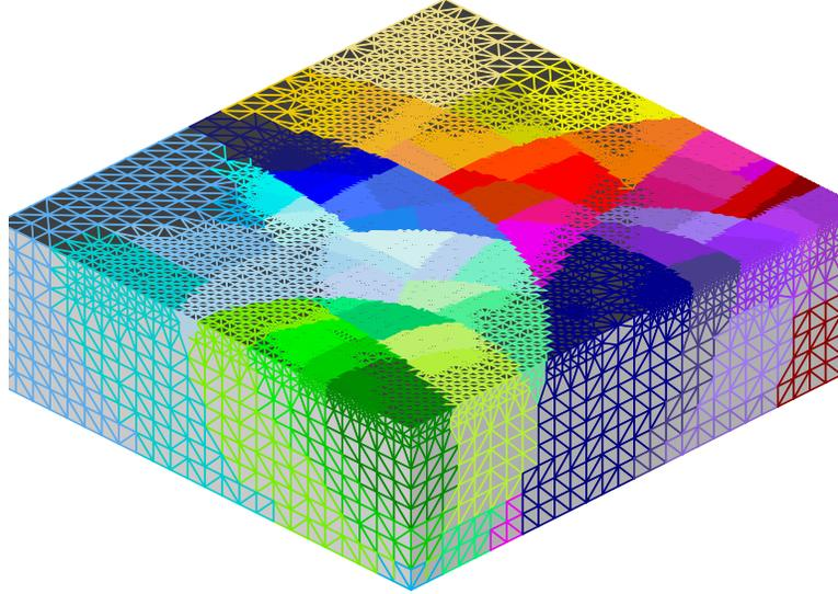
Figure 4: Mesh partitioned for 64 subdomains.
