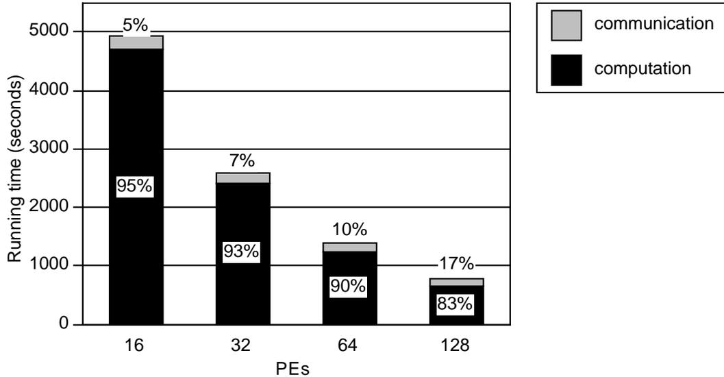
**Figure 8: Timings in seconds on a Cray T3D as a function of number of processors (PEs), excluding I/O. The breakdown of computation and communication is shown. The mesh is  $\mathcal{S}f2$ , and 6000 time steps are carried out.**
