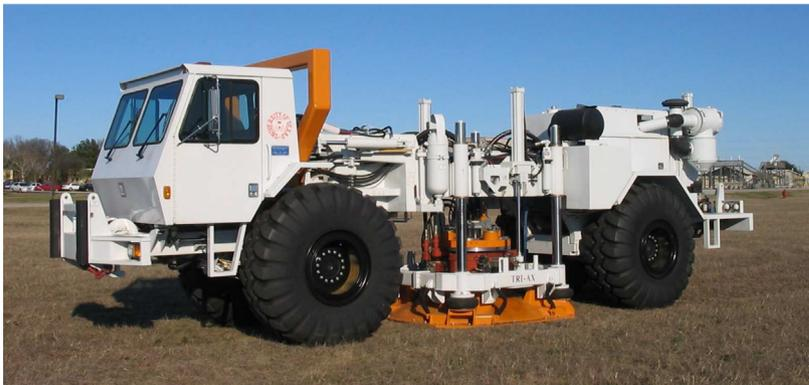
(a) NEES@UTexas T-Rex Vibroseis: the largest triaxial seismic vibration truck in the world
