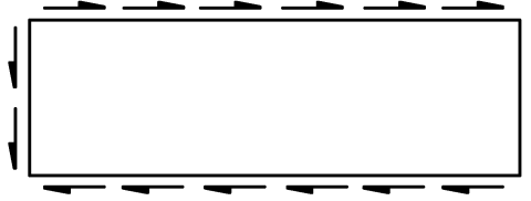
Figure 14.28–1 Uniform Shear on Rectangular Element
