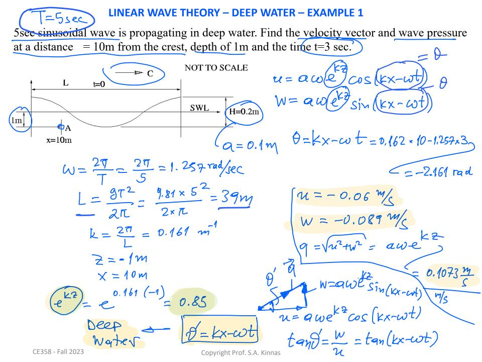
5sec sinusoidal wave is propagating in deep water. Find the velocity vector and wave pressure at a distance = 10m from the crest, depth of 1m and the time t=3 sec.
