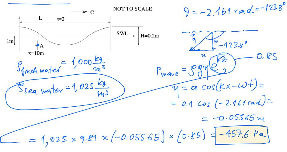
5sec sinusoidal wave is propagating in deep water. Find the velocity vector and wave pressure at a distance = 10m from the crest, depth of 1m and the time t=3 sec.
