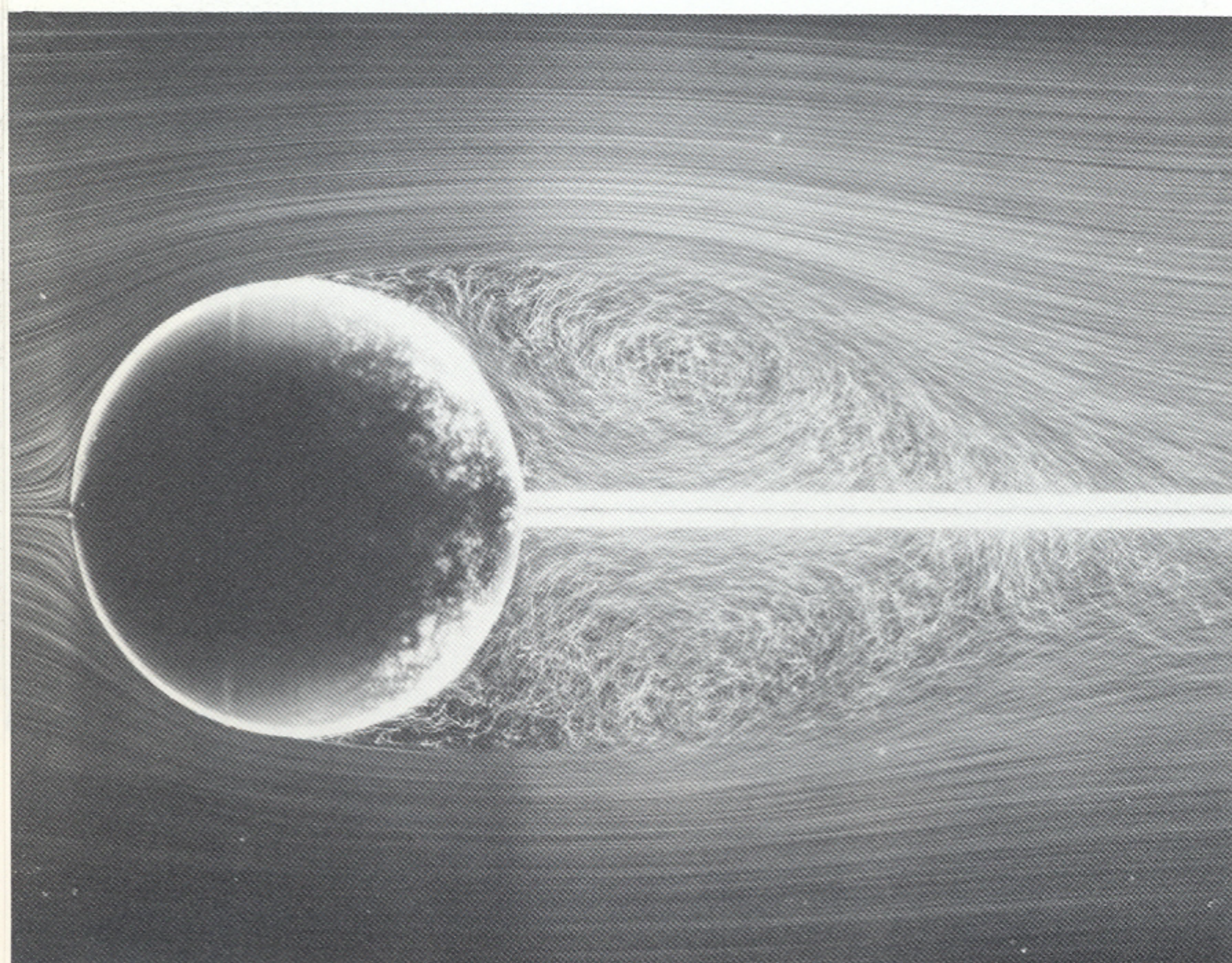
56. Mean flow past a sphere at R=15,000 . A time exposure of air bubbles in water shows an averaged streamline pattern in the meridian plane for the flow that was photographed instantaneously above. ONERA photograph by Henri Werlé
