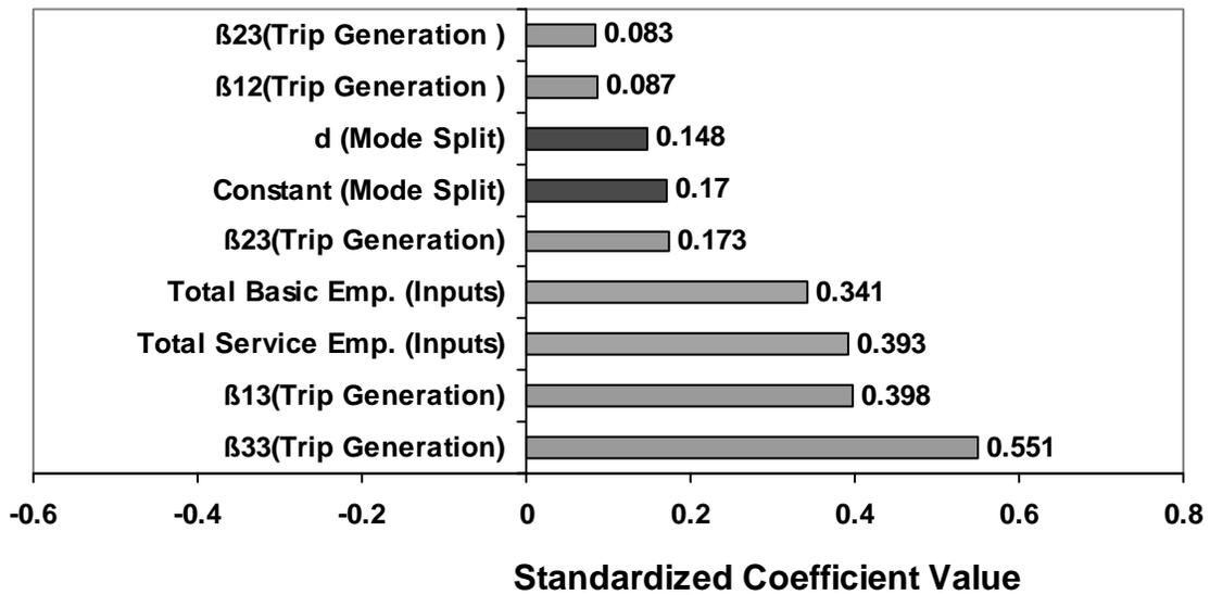
**Figure 7. Regression-based sensitivity analysis for final outputs**
