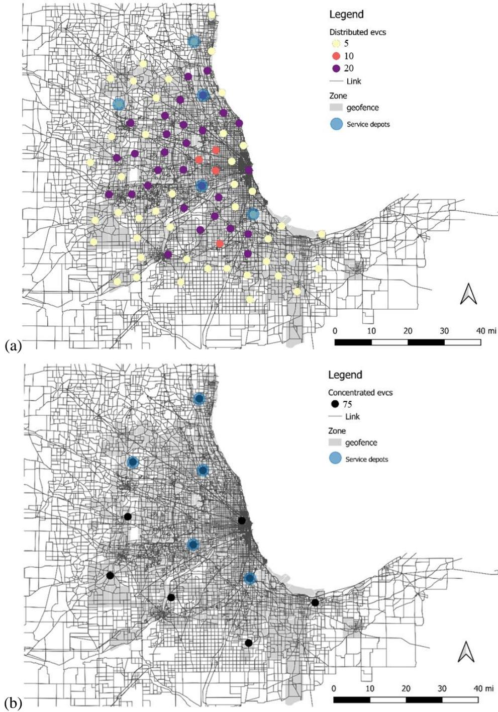
Figure 4 Chicago Road Networks with EVCS Locations (a – Distributed, b – Concentrated) and Sizing by Plug Count
