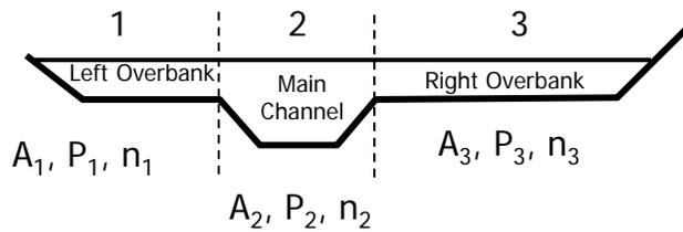
$$Q = \frac{\phi}{n} A R_h^{2/3} S^{1/2} = \sum_i \frac{\phi}{n_i} A_i R_{hi}^{2/3} S^{1/2}$$
