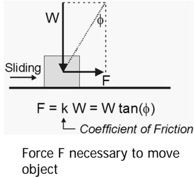
$\phi = \text{Angle of Repose}$
