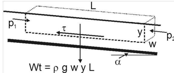
Force balance in downstream direction:
