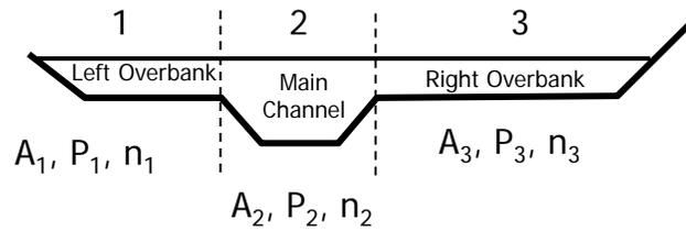
$$\alpha \frac{\bar{V}^2}{2g} = \frac{\sum_i Q_i (\alpha_i V_i^2 / 2g)}{\sum_i Q_i} \longrightarrow \alpha = A^2 \frac{\sum_i (\alpha_i K_i^3 / A_i^2)}{\left(\sum_i K_i\right)^3}$$
