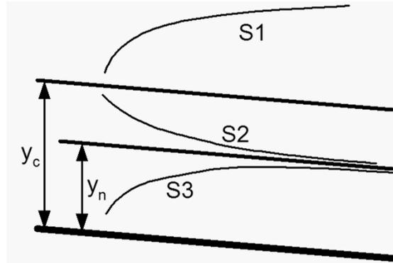
Note that for curves S2 and S3 the depth approaches normal depth in the direction for flow computation for supercritical flow
