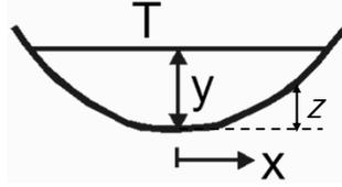
$$z = ax^2 \quad ; \quad T = 2\sqrt{\frac{y}{a}} \quad ; \quad A = \frac{4}{3}\sqrt{\frac{1}{a}}y^{3/2} = \frac{2}{3}Ty$$
