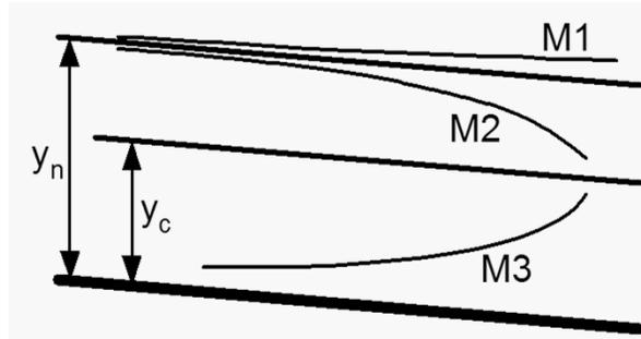
Note that for the M1 and M2 curves, the depth approaches normal depth in the direction of flow computation for subcritical flow.
