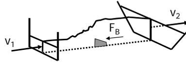
Momentum Equation:  $\Sigma F = \rho Q (V_2 - V_1)$
