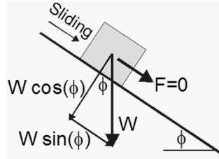
$$\frac{\text{Tangent}}{\text{Normal}} = \frac{W \sin(\phi)}{W \cos(\phi)} = \tan(\phi) = k$$
