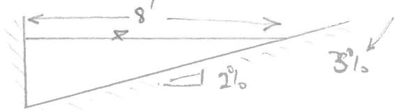
(b) Under these conditions if the flow in the gutter is 1.5 cfs, what percentage of the flow would be captured by a 10 ft curb inlet on grade?
