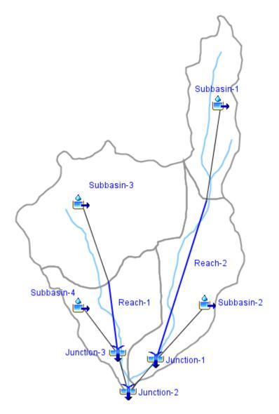
*Figure 30.* Subbasin, reach, and junction elements in their correct positions.
