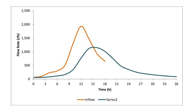
2. Problem # 8.4.4 A 4400-foot reach of channel has a Muskingum K=0.24 and X=0.25. Route the following inflow hydrograph through this reach. Assume the initial outflow =739cfs.
