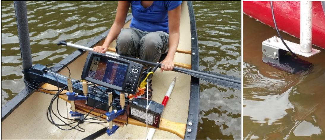
Figure 3. Images of the mounting process and orientation of the Humminbird.
