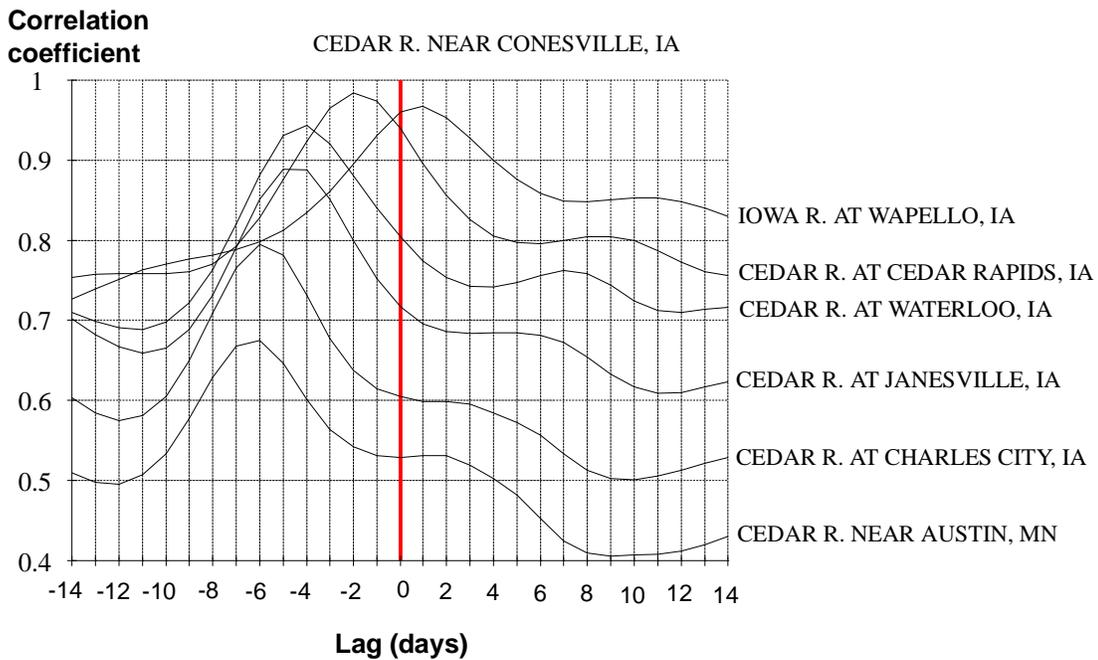
**Figure 4.21 Cross-correlation coefficients: the strength of the linear relationship between the flow rate in the Cedar River recorded near Conesville, IA, and the flow rate recorded at indicated locations. All gauging stations are on one flow path (shown in Figure 4.20).**
