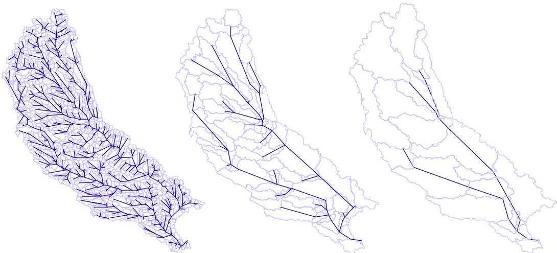
**Figure 4.12** Flow system in the Iowa-Cedar River basin subdivided into modeling units of different sizes (threshold drainage area: 25 km<sup>2</sup>, 400 km<sup>2</sup>, and 2500 km<sup>2</sup>).
