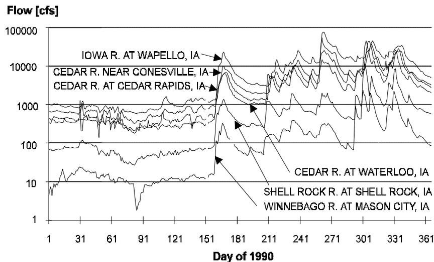
**Figure 4.19** Example of time series recorded in gauging stations located along the Cedar River. The data are for the water year 1990. The logarithmic scale is used to show all time series in one picture.
