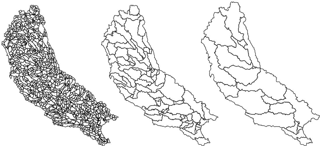
**Figure 4.10** Division of the Iowa-Cedar River into modeling units using different threshold drainage areas: 25 km<sup>2</sup>, 400 km<sup>2</sup>, and 2500 km<sup>2</sup>.
