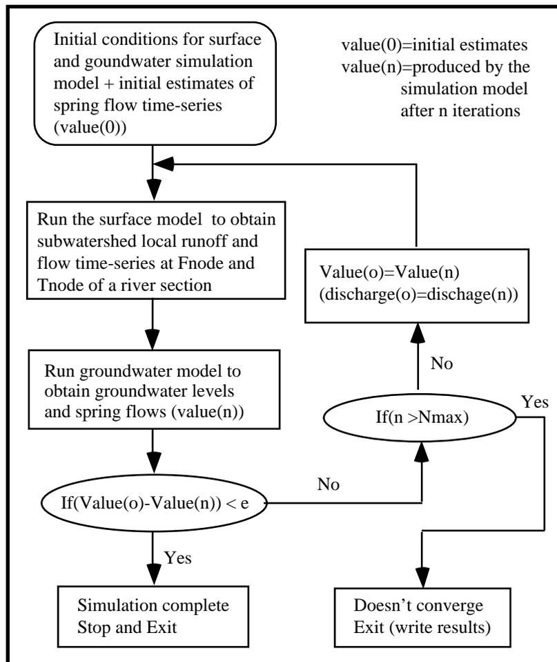
Figure 5.3. Simulating procedure of an integrated model
