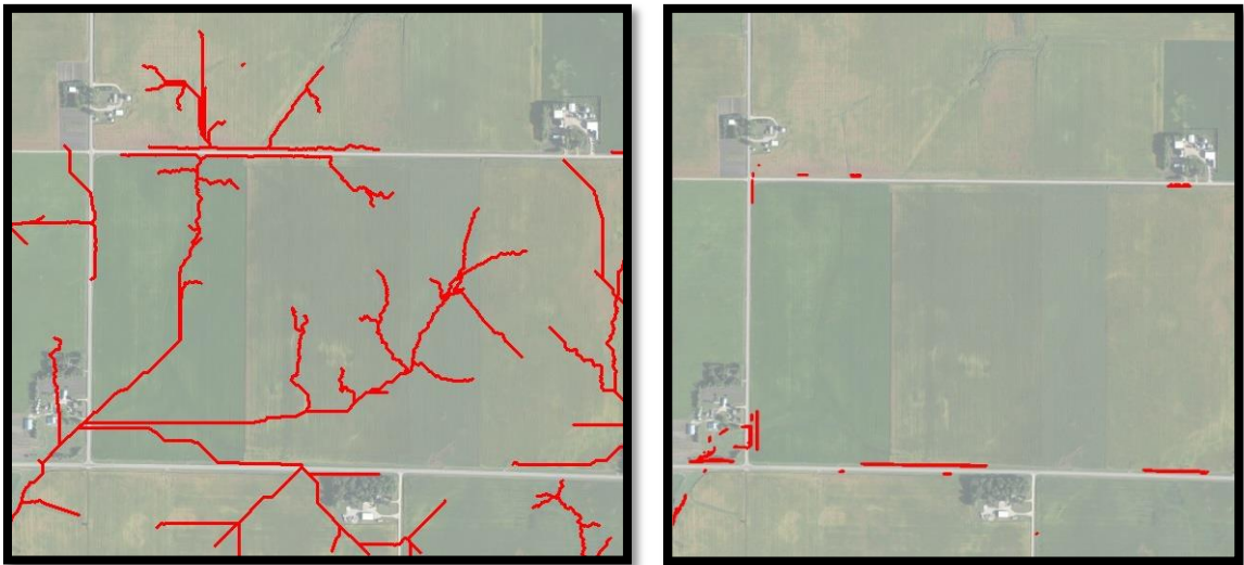
Figure 24. Roads extracted as channel features in Le Seuer sub-basin by (a) ArcMap and (b) GeoNet.
