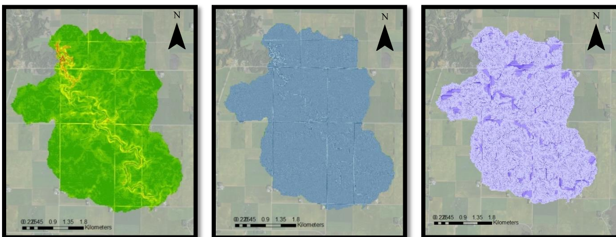
Figure 8. From left to right: slope, curvature, and accumulation area rasters for Le Seuer sub-basin.
