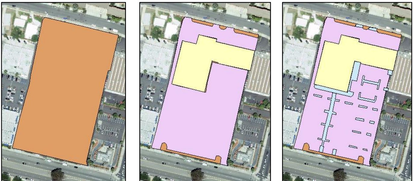
Figure 7: Polygon of the entire SGD&E property (brown). Polygon of the impervious roof (yellow). Polygon of the impervious asphalt (pink). Polygons of the pervious LID (blue). The middle image represents pre-LID conditions and the right reflects post-LID conditions.
