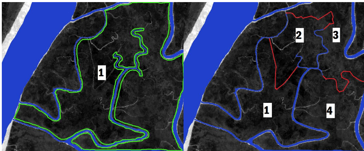
Figure 12: Image of the island network with and without manual channel connections. Green lines represent the model interpretation. Red lines represent connections that can be seen in ground truth data.
