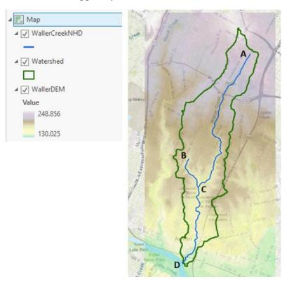
The file austin.zip provided for problem 3 includes a 10 m digital elevation model (DEM) for this area obtained from the National Map (WallerDEM) and the NHD streams within the Waller Creek Watershed, both projected into UTM coordinates.
