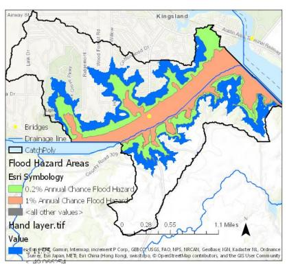
Figure 9. National Flood Hazard Layer and HAND flood depth
