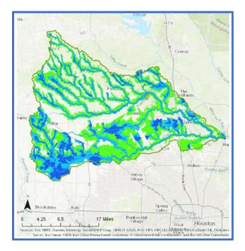
Figure 8: Height Above Nearest Drainage for entire basin.
