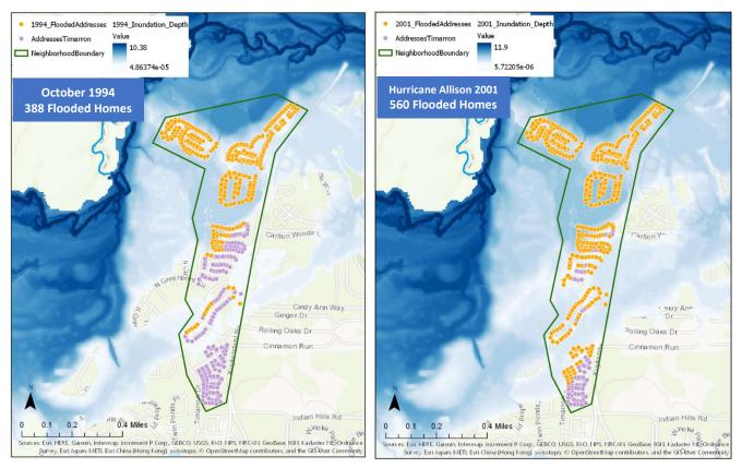
Figure 11: Left – October 1994 Inundation Map. Right – Hurricane Allison 2001 Inundation Map.
