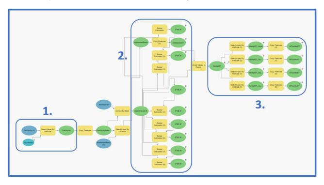
Figure 9: Model Builder used to determine inundation depths and flooded addresses.
