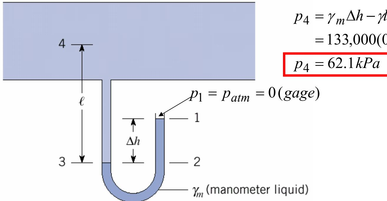
$$\begin{aligned} p_4 &= \gamma_m \Delta h - \gamma l \\ &= 133,000(0.6) - 9810(1.8) \end{aligned}$$
