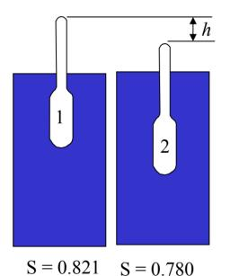
A hydrometer weighs 0.0216 N and has a stem at the upper end that is cylindrical and 2.8 mm in diameter.
