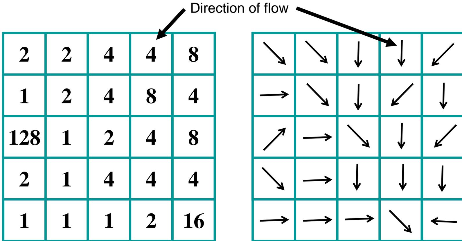
Part of a Digital Elevation Model
