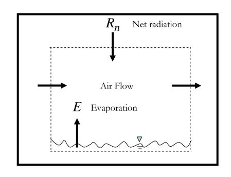
$$\frac{\dot{m}}{\tau} = \frac{K_w (q_{v_1} - q_{v_2})}{K_m (u_2 - u_1)}$$
