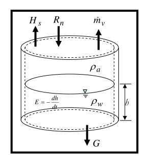
$$-\dot{m}_{v} = \frac{d}{dt} \iiint_{CV} \rho_{w} d \forall + \iint_{CS} \rho_{w} V \cdot dA$$
