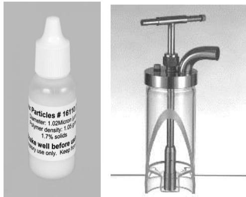
Figure 3-4: Latex particle solution and Collison Nebulizer particle generator
