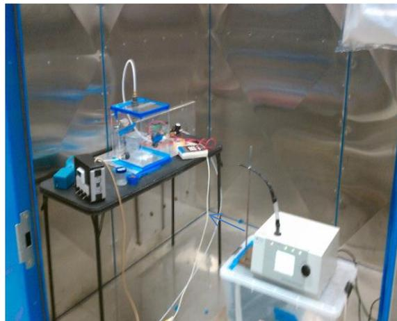
Figure 3-3: The small cubic chamber for experiments related to coughing
