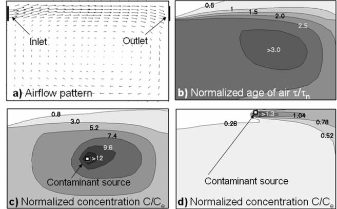
**Figure 2** Normalized local age of air and contaminant concentration distributions for the same airflow field and different positions of the contaminant source; (a) airflow pattern, (b)  $\epsilon_a = 0.21$  for this airflow pattern, (c)  $\epsilon_a = 0.21$  and  $\epsilon = 0.19$  for contaminant source at room center, (d)  $\epsilon_a = 0.21$ , and  $\epsilon = 2.20$  for contaminant source in the supply air jet.
