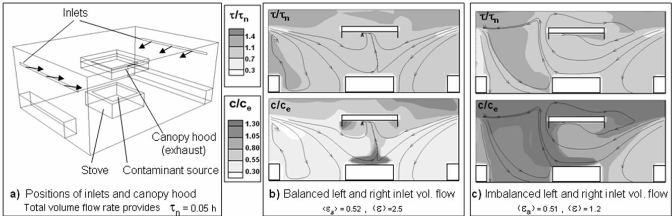
**Figure 8** Air exchange efficiency ( $\epsilon_a$ ) and contaminant removal effectiveness ( $\epsilon$ ) in the kitchen for: balanced flow—left and right inlet volume flow rate are the same; imbalanced flow—left inlet volume flow rate is one-third of right.
