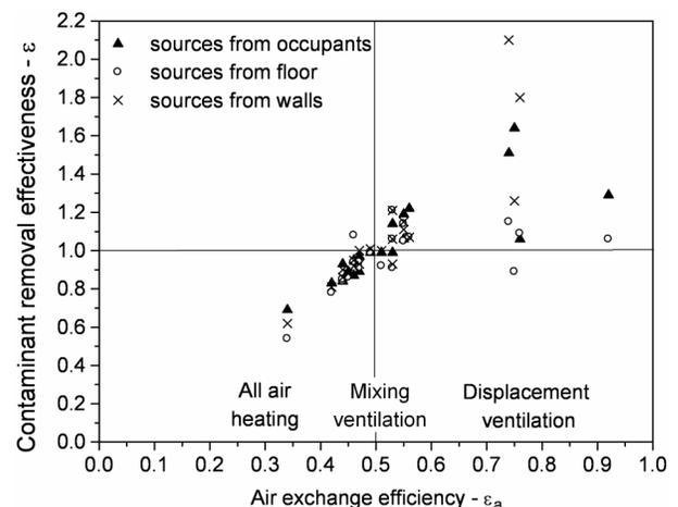
Figure 6 The correlation between air exchange efficiency and contaminant removal effectiveness.
