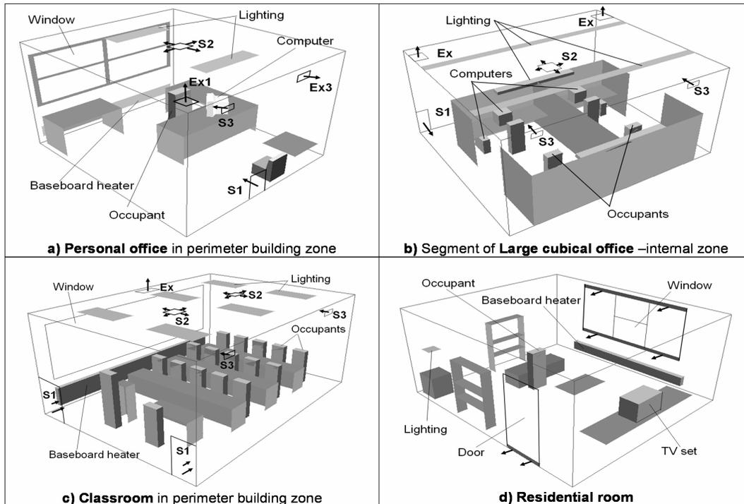
**Figure 3** Space layouts with supply and exhaust positions for the analyzed cases (S1 – displacement ventilation diffuser, S2 – ceiling mixing diffuser, S3 – grille diffuser, Ex – exhaust).
