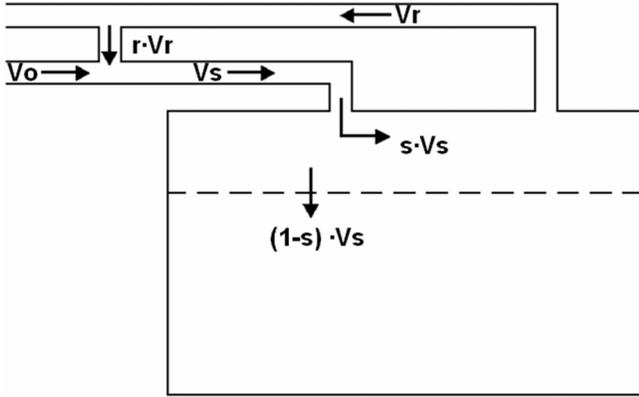
**Figure 1** The two-zone model used to define ventilation effectiveness  $E_v$  (ASHRAE 2001).
