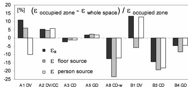
**Figure 5** Differences in air exchange efficiency ( $\epsilon_a$ ) and contaminant removal effectiveness defined for the occupied zone ( $\epsilon_{\text{occupied zone}}$ ) and the entire space ( $\epsilon_{\text{whole space}}$ ).
