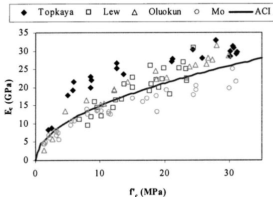
Fig. 12. Concrete stiffness test results
