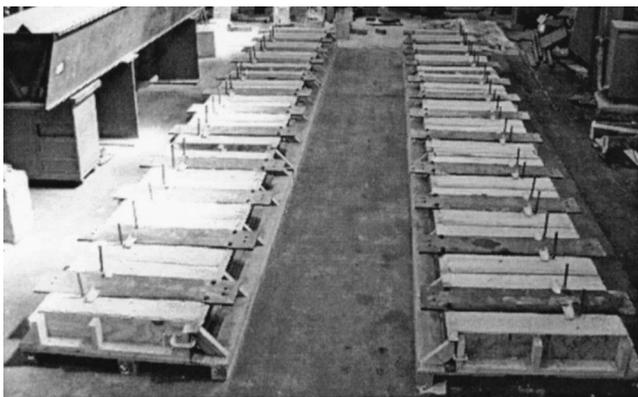
**Fig. 5.** View of all pushout test specimens
