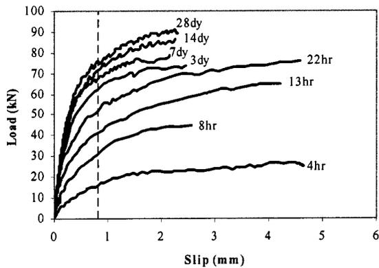
Fig. 7. Load-slip relationship from pushout tests
