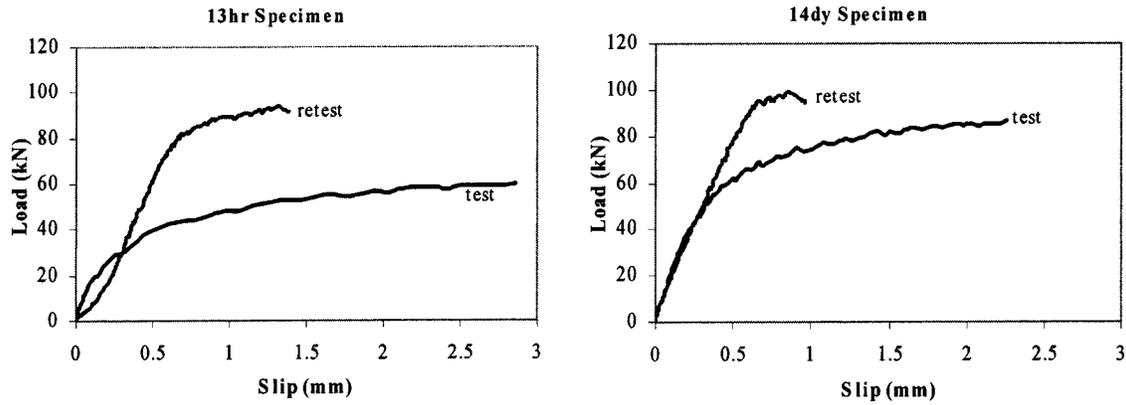
Fig. 14. Load-slip behavior of retested specimens
