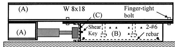
Fig. 3. Schematic of pushout test setup
