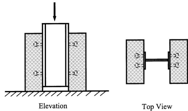
Fig. 1. Conventional pushout test setup
