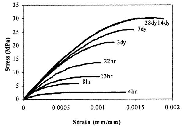
Fig. 10. Compressive stress-strain response
