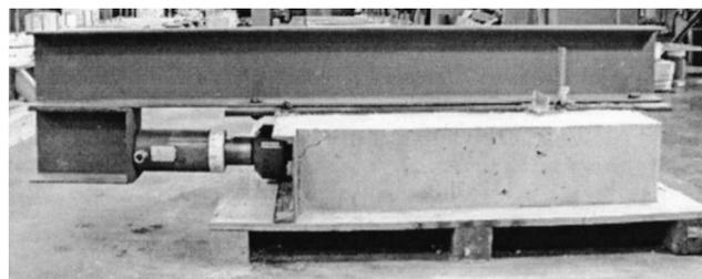
Fig. 4. Side view of pushout test setup
