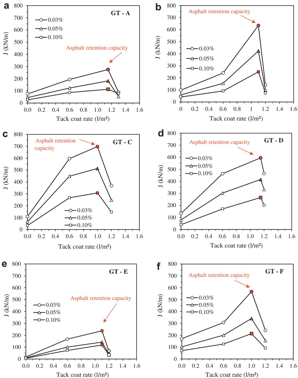
**Fig. 8.** Stiffness curves (J) versus tack coat rate at different strain levels for paving geotextiles: (a) GT-A; (b) GT-B; (c) GT-C; (d) GT-D; (e) GT-E and (f) GT-F.
