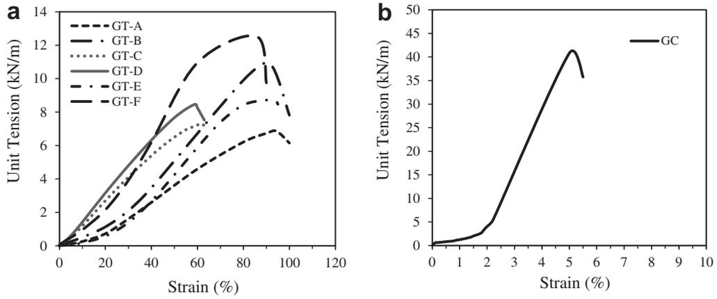
**Fig. 3.** Unit tension–strain curves for the geotextiles tested in the cross-machine direction: (a) nonwoven geotextiles; (b) geogrid composite.
