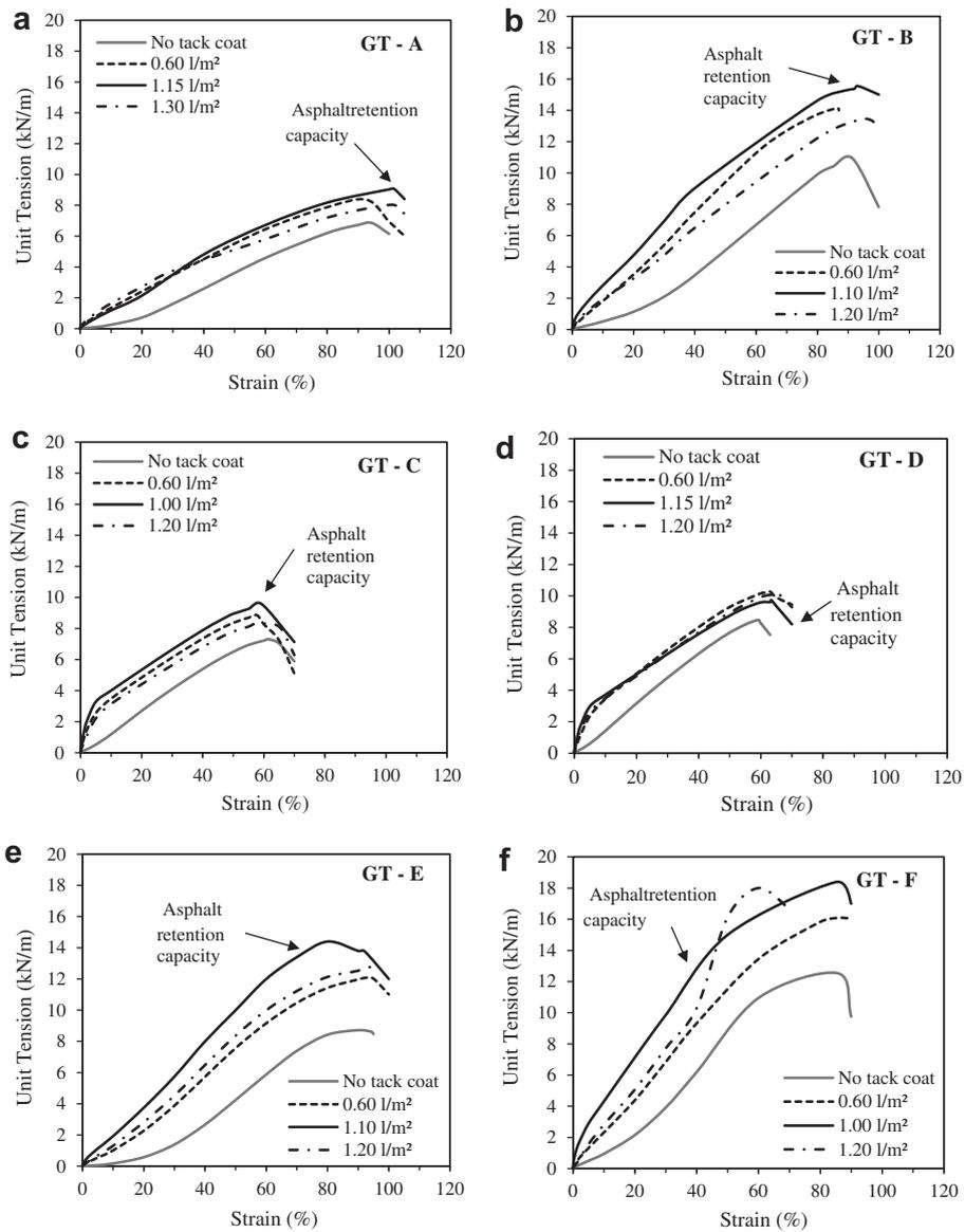
**Fig. 4.** Unit tension–strain curves of nonwoven geotextiles impregnated with different rates of emulsion: (a) GT-A; (b) GT-B; (c) GT-C; (d) GT-D; (e) GT-E and (f) GT-F.
