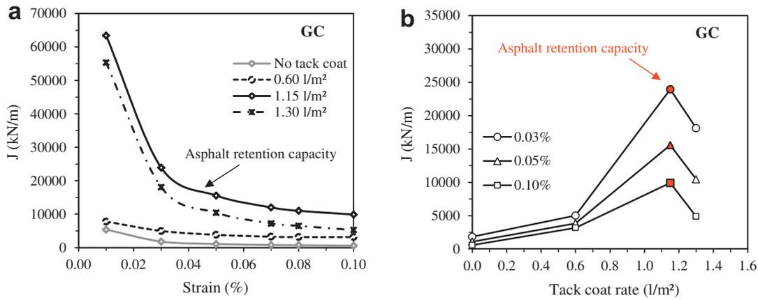
Fig. 9. Tensile results for geogrid composite: (a) stiffness curves versus percentage strain with different rates of asphalt emulsion; (b) increase in the UTS as function of tack coat rate.
