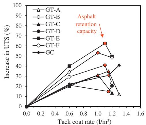
Fig. 6. Increase in the UTS as function of tack coat rate for the geosynthetic paving materials used in this study.
