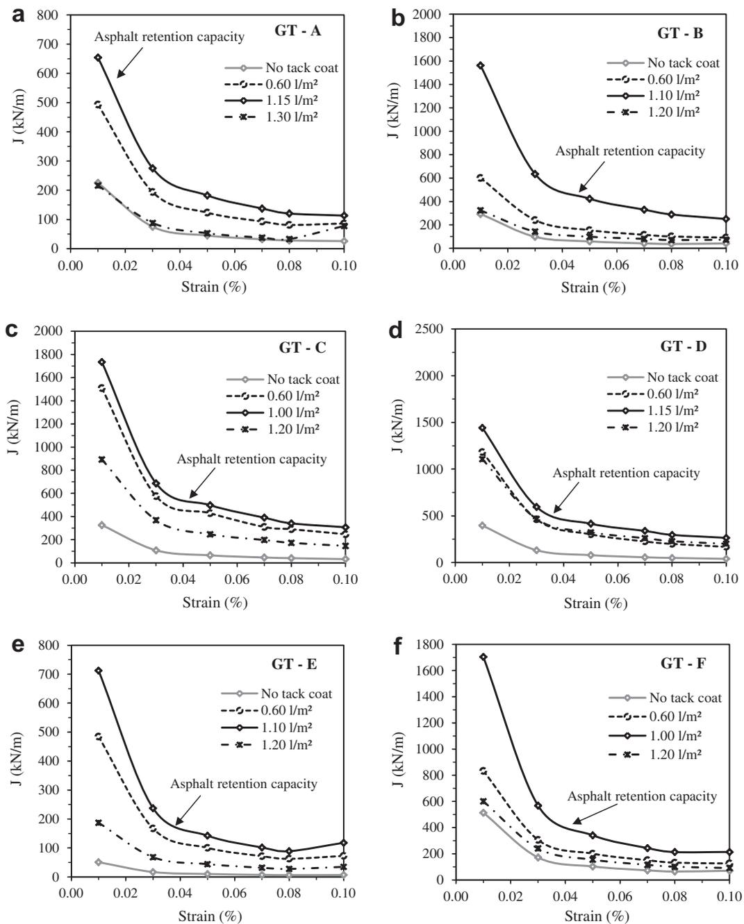
**Fig. 7.** Stiffness curves ( $J$ ) versus percentage strain for paving geotextiles with different rates of asphalt emulsion: (a) GT-A; (b) GT-B; (c) GT-C; (d) GT-D; (e) GT-E and (f) GT-F.
