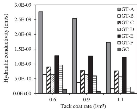
Fig. 11. Hydraulic conductivity as function of tack coat rate for the geosynthetic paving materials used in this study.
