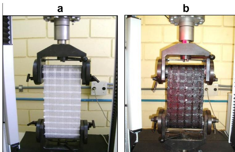
**Fig. 2.** View of tensile tests in progress: (a) virgin geogrid composite; (b) geogrid composite impregnated with asphalt emulsion.
