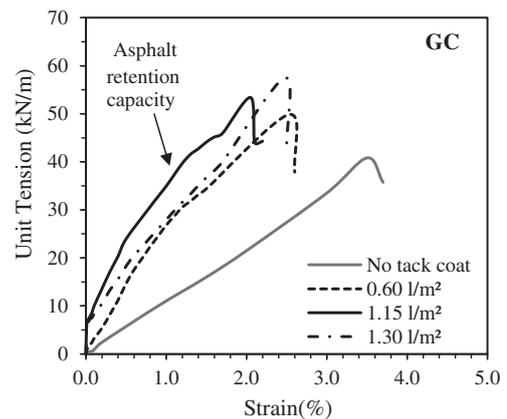
Fig. 5. Unit tension-strain curves of geogrid composite impregnated with different rates of emulsion.
