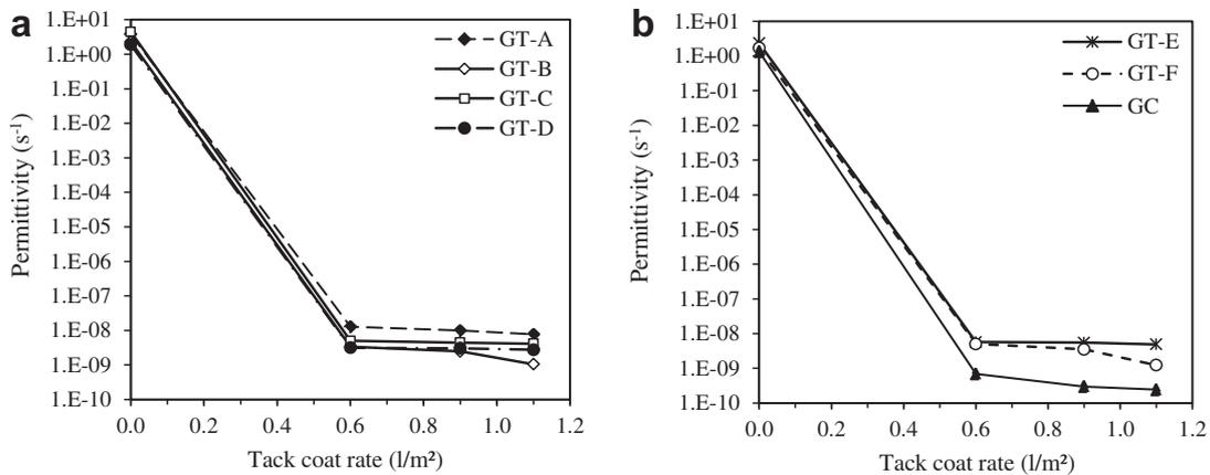
Fig. 10. Permittivity values of impregnated geosynthetics with different rates of emulsion: (a) PET nonwoven geotextiles; (b) PP nonwoven geotextiles and geogrid composite.
