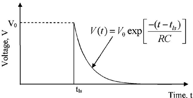
Fig. 6. Response of the analogous model of the water content reflectometer system to a lightning strike at time  $t_{ls}$ .
