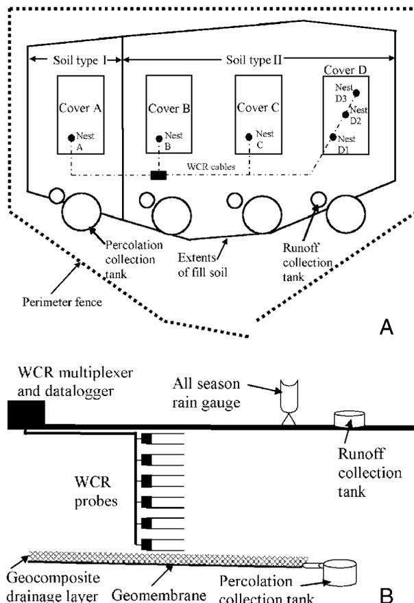
Fig. 2. Layout for the monitoring program at the Rocky Mountain Arsenal: (A) plan view; (B) elevation view.
