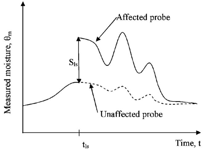
**Fig. 4. Schematic representation of the effect of a lightning strike;  $t_{Is}$  is the time of the strike and  $S_{Is}$  is the shift in the moisture content reading induced by the strike.**
