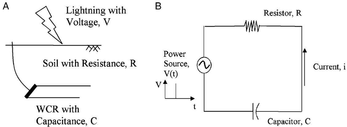
Fig. 5. Conceptualization of the water content reflectometer system in the event of a lightning strike: (A) physical model; and (B) analogous model.
