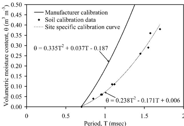
Fig. 1. Water content reflectometer calibration curve for the Rocky Mountain Arsenal soils.
