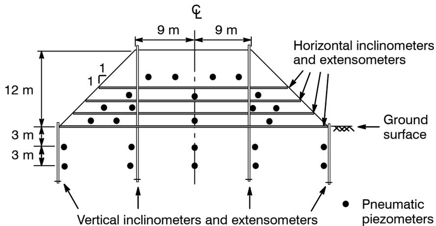
**Figure 3. Instrumentation in Devon test fill (after Scott et al. 1987).**
