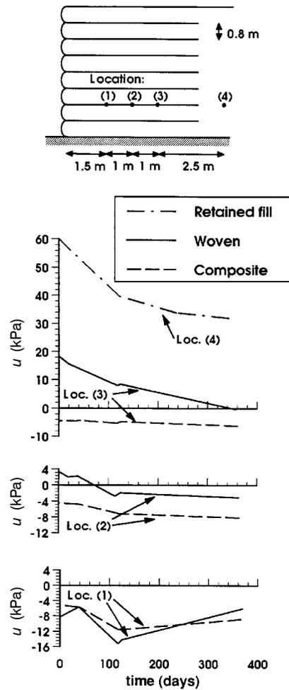
**Figure 5. Porewater pressures ( $u$ ) recorded in the Rouen reinforced wall, along a woven and a nonwoven/geogrid composite, at different locations within the silty backfill (redrawn after Perrier et al. 1986).**
