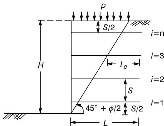
**Figure 7. Arrangement of reinforcements in a clay wall model (after Ingold 1981).**
