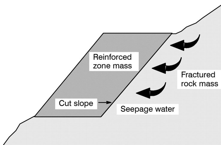
Figure 17. Water infiltration in a reinforced slope for road widening projects.
