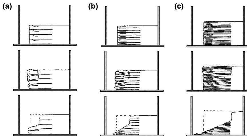
**Figure 11.** Sequence of failure for centrifuge models of kaolin clay reinforced with nonwoven geotextiles: (a) lightly reinforced model; (b) intermediate reinforced model; (c) heavily reinforced model (after Goodings 1990).
