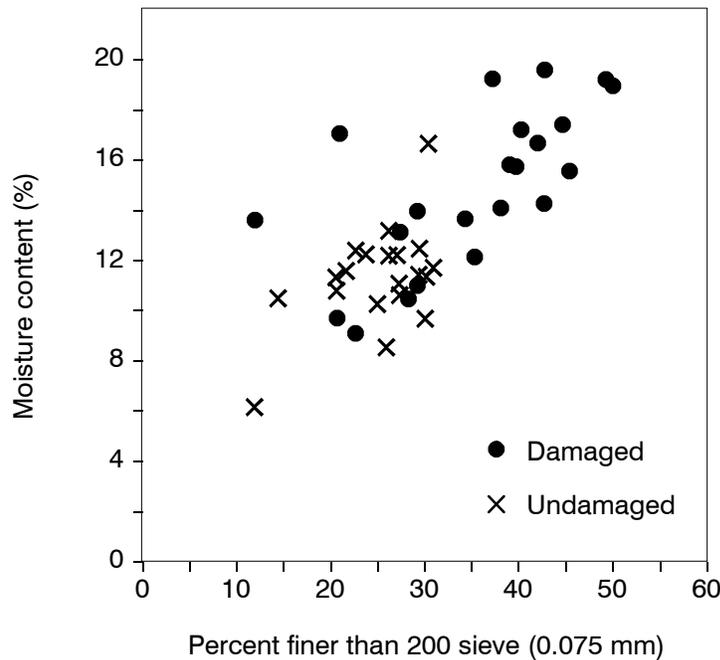
**Figure 8. Moisture content and percentage fines for damaged and undamaged walls reinforced with metallic strips (after Elias and Swanson 1983).**
