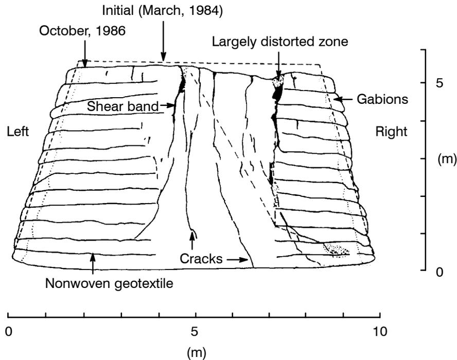
**Figure 12.** Cross-section of clay Test Embankment II, observed at dismantling (after Yamauchi et al. 1987).
