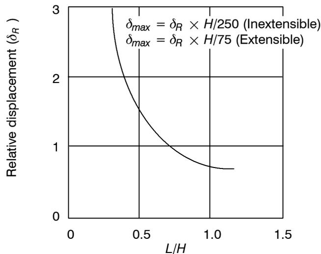
**Figure 14. Curve for estimation of lateral displacement anticipated at the end of construction of reinforced walls (after Mitchell and Christopher 1990).**
