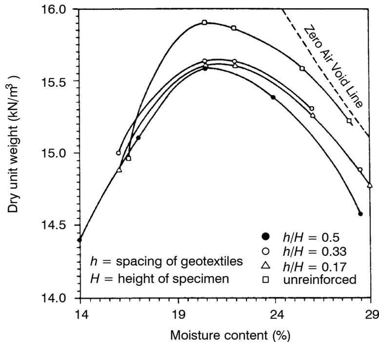
**Figure 19.** Effect of nonwoven geotextile spacing on compaction curves for reinforced clay specimens (after Indraratna et al. 1991).
