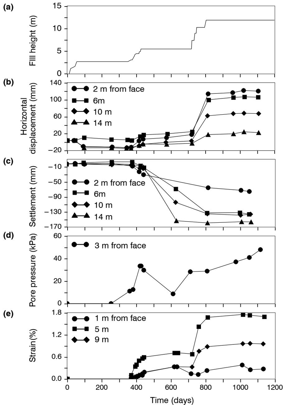
**Figure 4.** Field measurements at 3 m above base and at various distances from slope face within embankment and geogrids of Devon test fill: (a) fill height; (b) horizontal displacements; (c) settlements; (d) pore pressures; (e) geogrid strains (after Sego et al. 1990).
