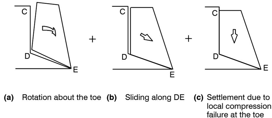
**Figure 13.** Schematic diagram showing deformation of right-hand slope of Test Embankment II in Figure 12 (after Yamauchi et al. 1987).
