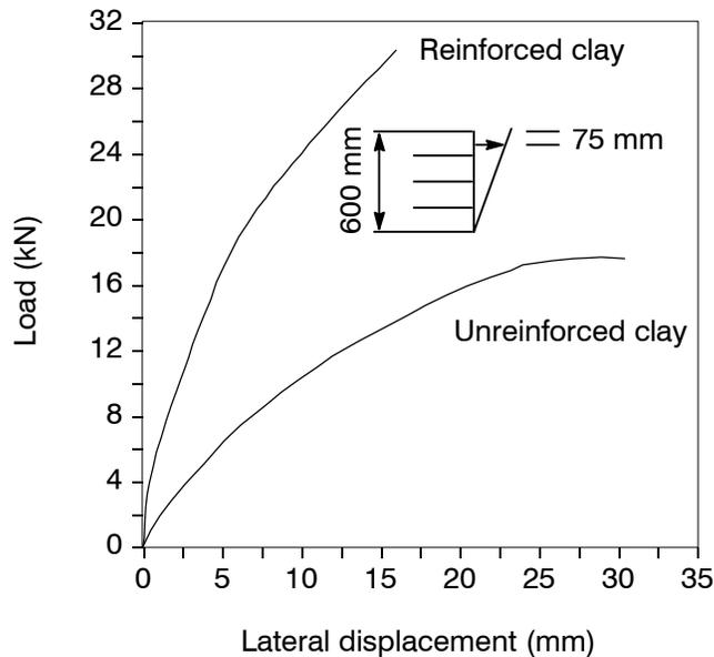
**Figure 15. Load-horizontal displacement curves of reinforced and unreinforced clay wall models (after Fabian and Fourie 1988).**
