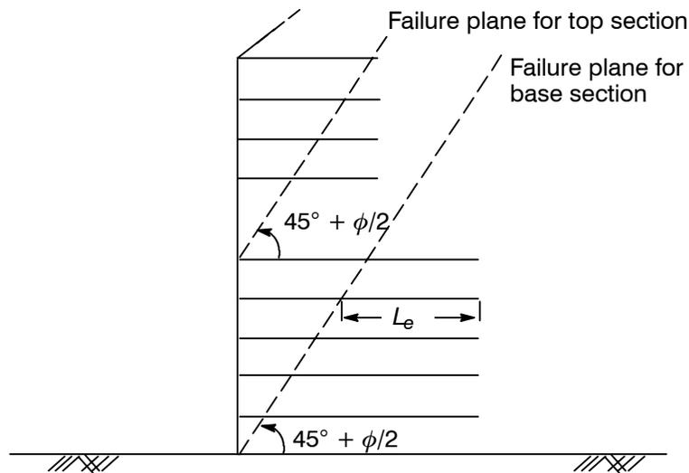
**Figure 9. Configuration of welded wire wall on Interstate 580, California (after Mitchell and Villet 1987).**
