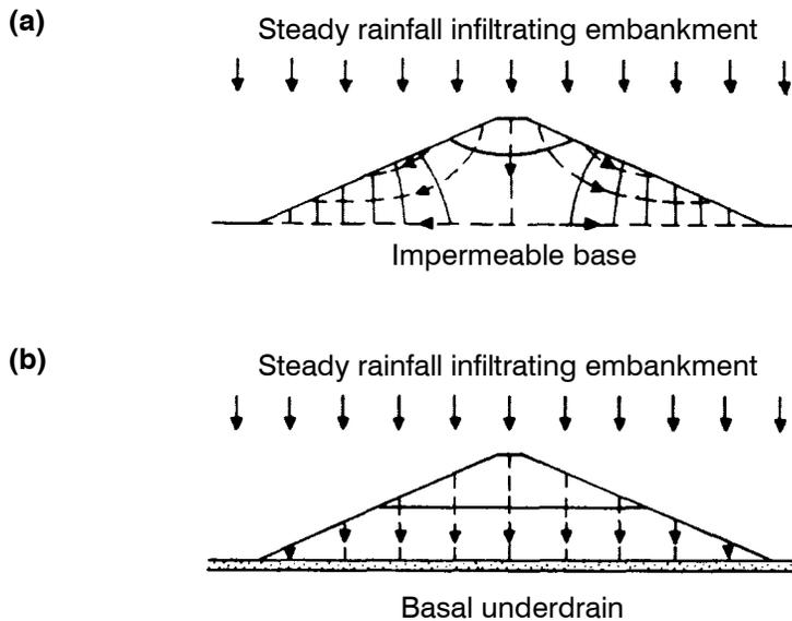
**Figure 18. Flow regime for embankment: (a) on an impermeable base; (b) on a pervious base (after Ingold 1992).**
