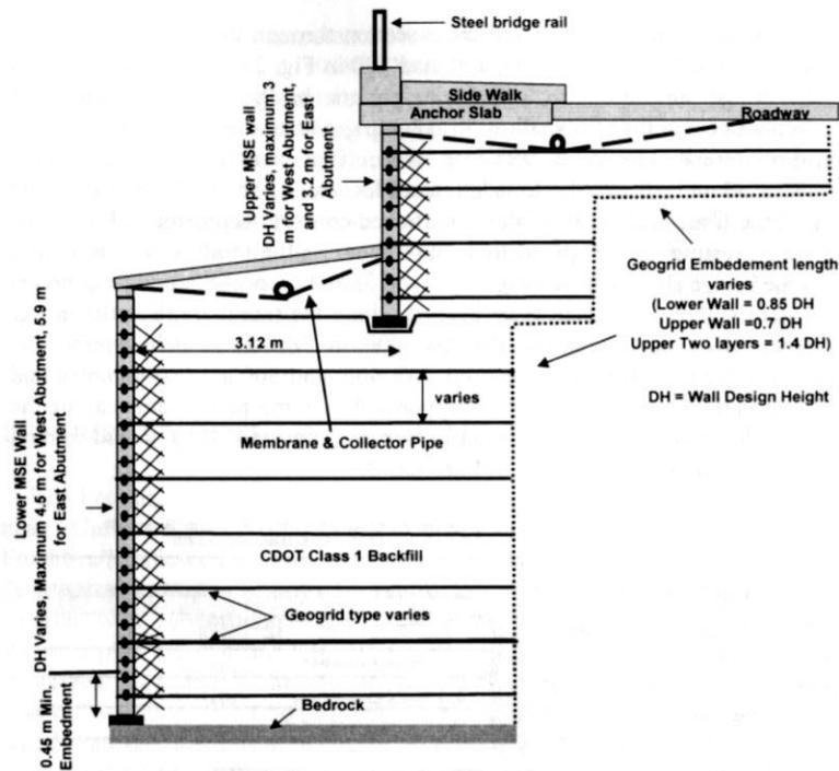
Fig. 4. Typical Cross-Section along the Upper and Lower MSE walls (e.g., Sections 300 and 900 in Fig. 2)
