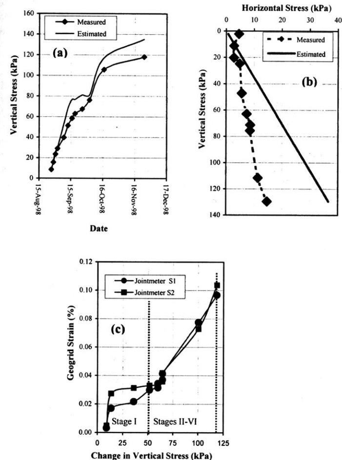
Fig. 7. Measured and Estimated Data on Section 400 of Phase I Structure: (a) Vertical Stresses, (b) Horizontal Stresses, and (c) Geogrid Strains.
