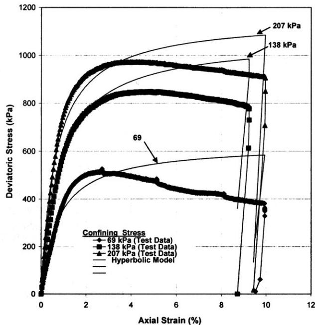
Fig. 5. Deviatoric Stress-Axial Strain Test Results from Large-Size Triaxial Tests and Predictions from Hyperbolic Model
