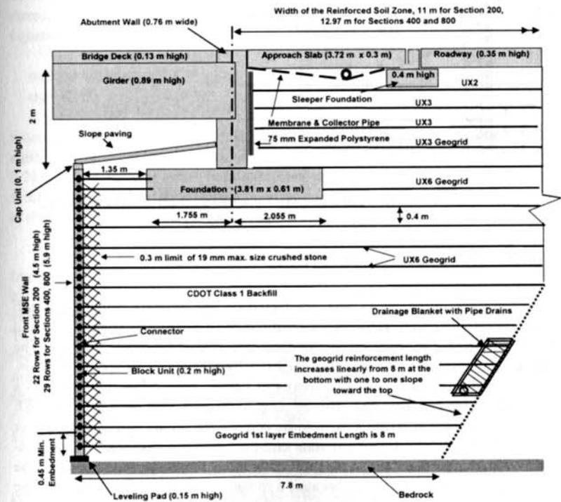
Fig. 3. Typical Monitored Cross-Section (Sections 200, 400, and 800 in Fig. 2) through the Front and Abutment MSE walls
