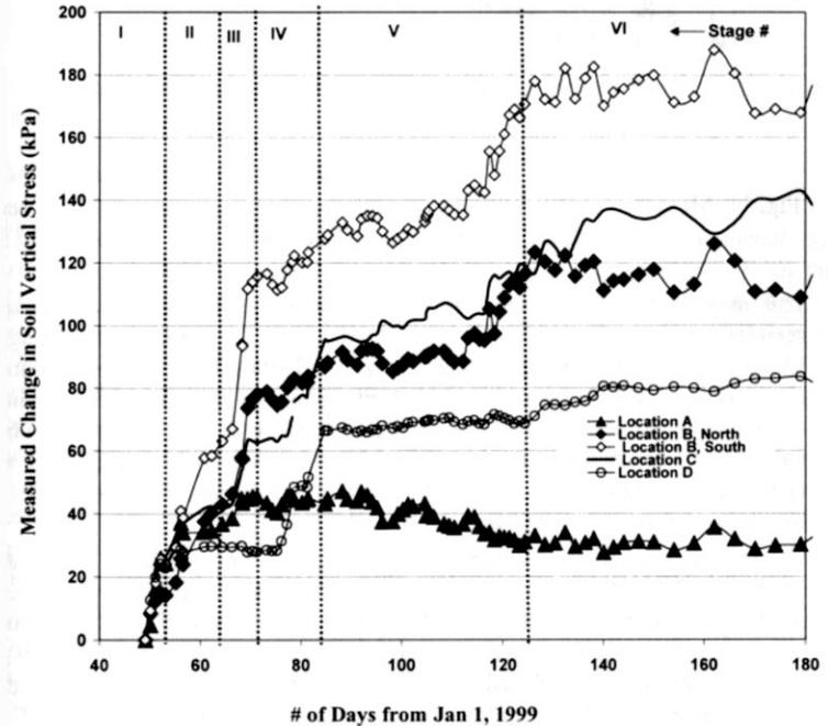
Fig. 10. Measured Vertical Soil Stresses during all Construction Stages (Measured between Geogrid Layers 10 and 11 along Section 800)
