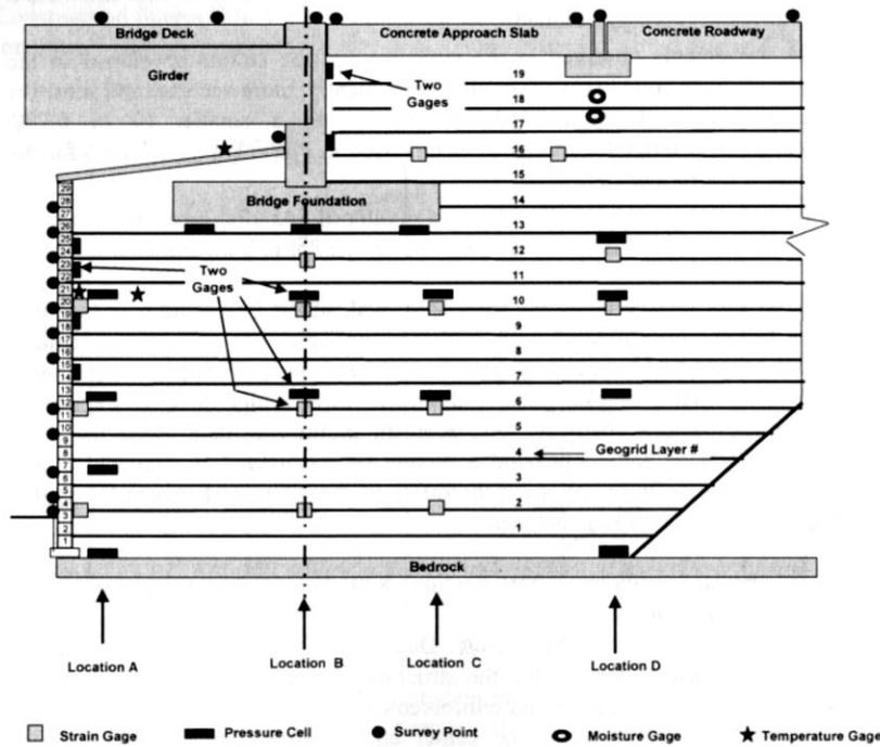
Fig. 9. Instrumentation Layout at Section 800 (Phase II structure)
