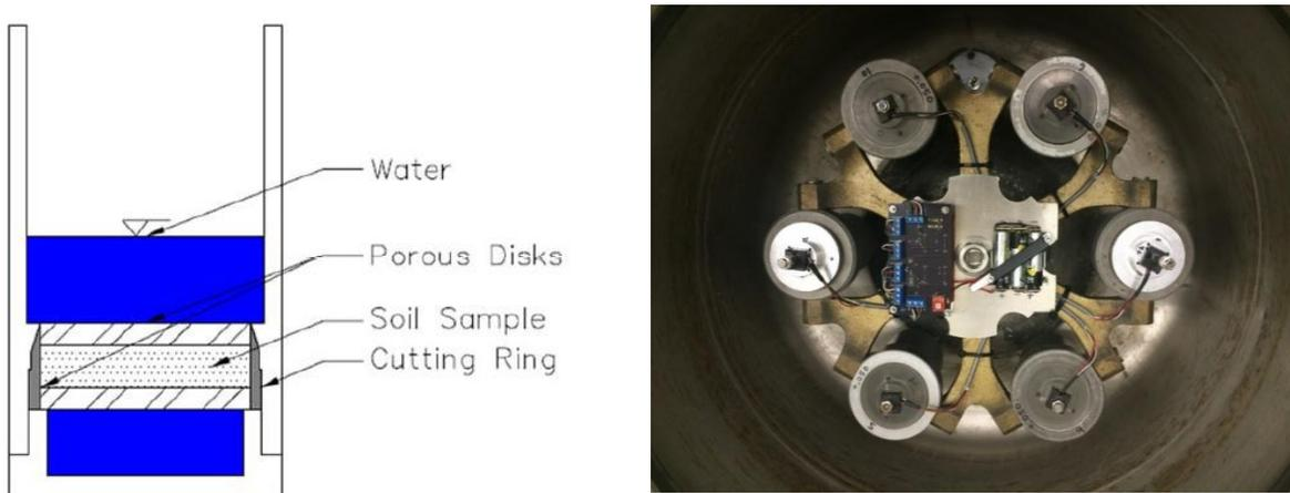
**Figure 1. Side view of permeameter cup (left) and overview of centrifuge system (right)**
